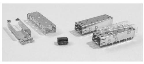
TE offers various termination options for SFP cages, including press-fit, wave solder and IR reflow compatible with tape and reel packaging. The connector is a reliable 20 position
