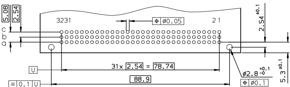
SPECIFICATION 893 = Grounding pins in position A1 & A32
