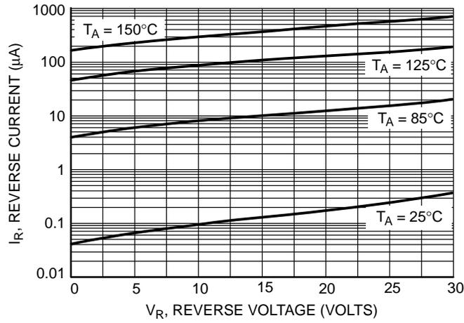
Figure 3. Leakage Current
