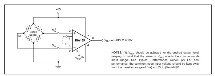
FIGURE 2. Single-Supply Bridge Amplifier.
