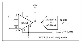
FIGURE 9. INA155 Directly Drives Capacitive-Input, High-Speed A/D Converter.
