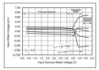
FIGURE 6. Input Offset Voltage Changes with Common-Mode Voltage.
