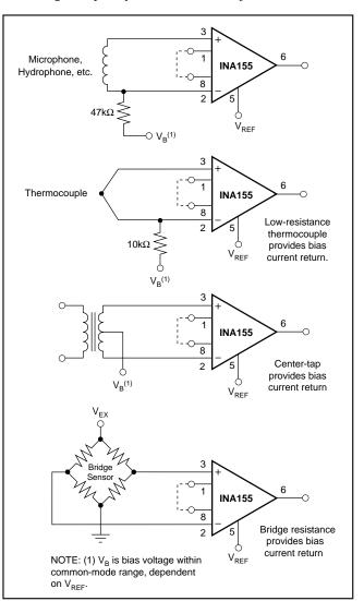
FIGURE 5. Providing an Input Common-Mode Current Path.
