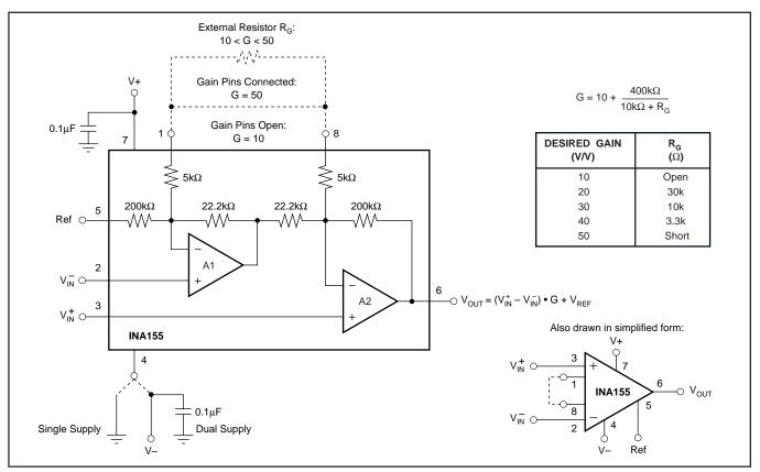
FIGURE 1. Basic Connections.
