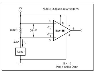
FIGURE 7. Single-Supply, High-Side Current Monitor.
