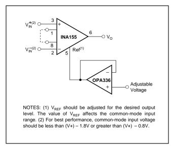
FIGURE 4. Optional Trimming of Output Offset Voltage.
