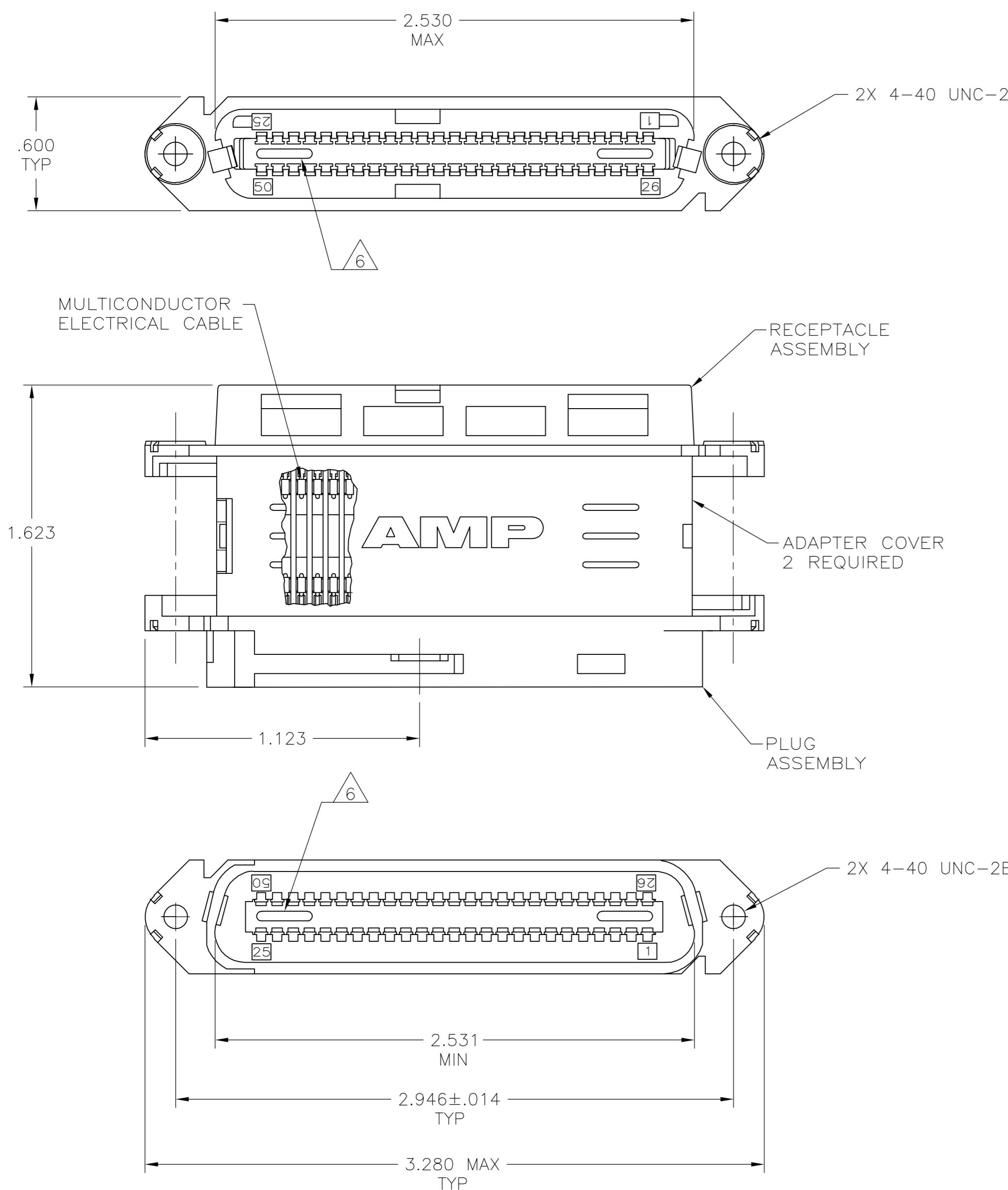
1. LIKE NUMBERED CONTACTS ON BOTH CONNECTORS ARE ELECTRICALLY COMMON.
