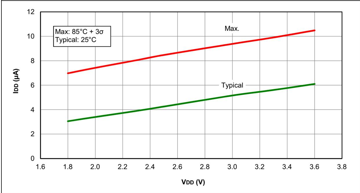
**FIGURE 28-14:  $I_{DD}$ , LFINTOSC,  $F_{osc} = 31$  kHz, PIC12F1501 ONLY**
