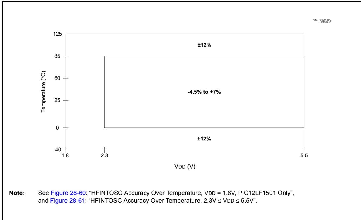
**Note:** See Figure 28-60: “HFINTOSC Accuracy Over Temperature, V<sub>DD</sub> = 1.8V, PIC12LF1501 Only”, and Figure 28-61: “HFINTOSC Accuracy Over Temperature, 2.3V ≤ V<sub>DD</sub> ≤ 5.5V”.
