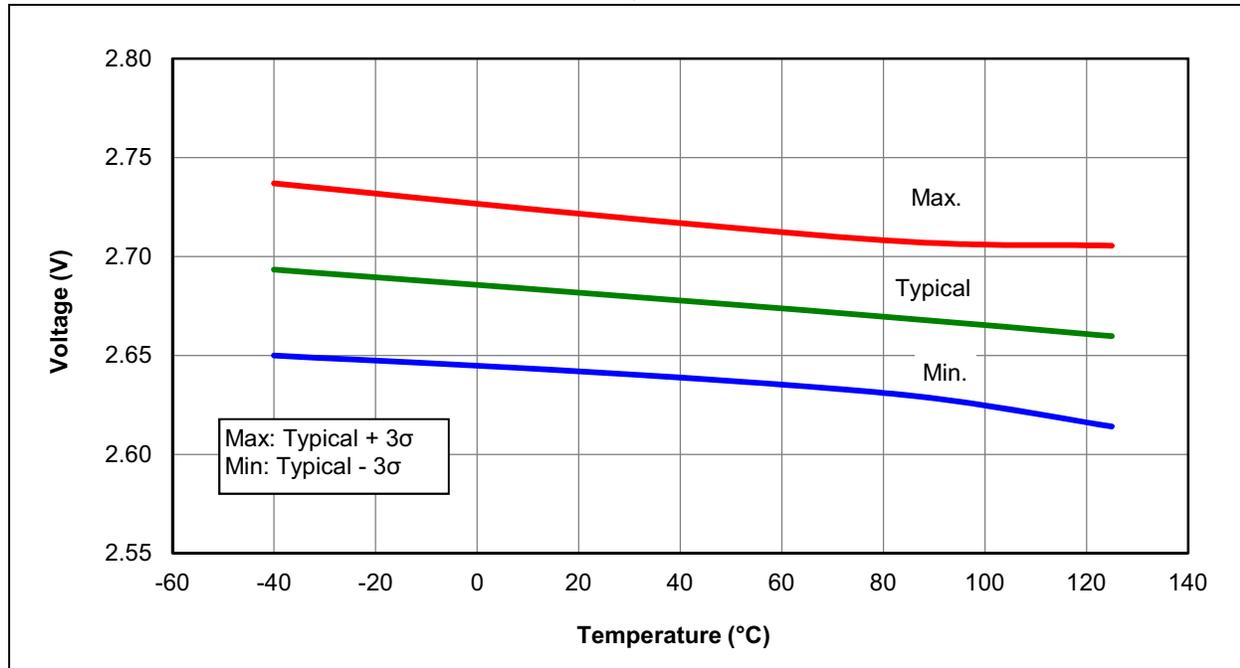
**FIGURE 28-48: LOW-POWER BROWN-OUT RESET VOLTAGE, LPBOR = 0**
