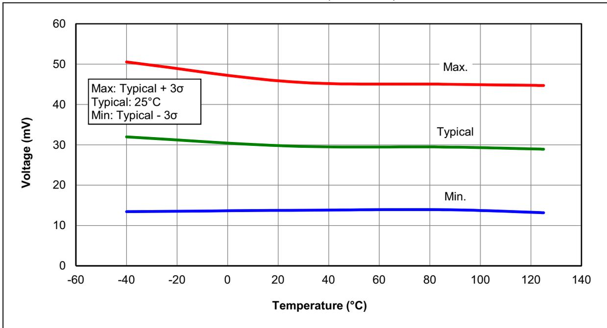
**FIGURE 28-45: BROWN-OUT RESET VOLTAGE, BORV = 1, PIC12F1501 ONLY**
