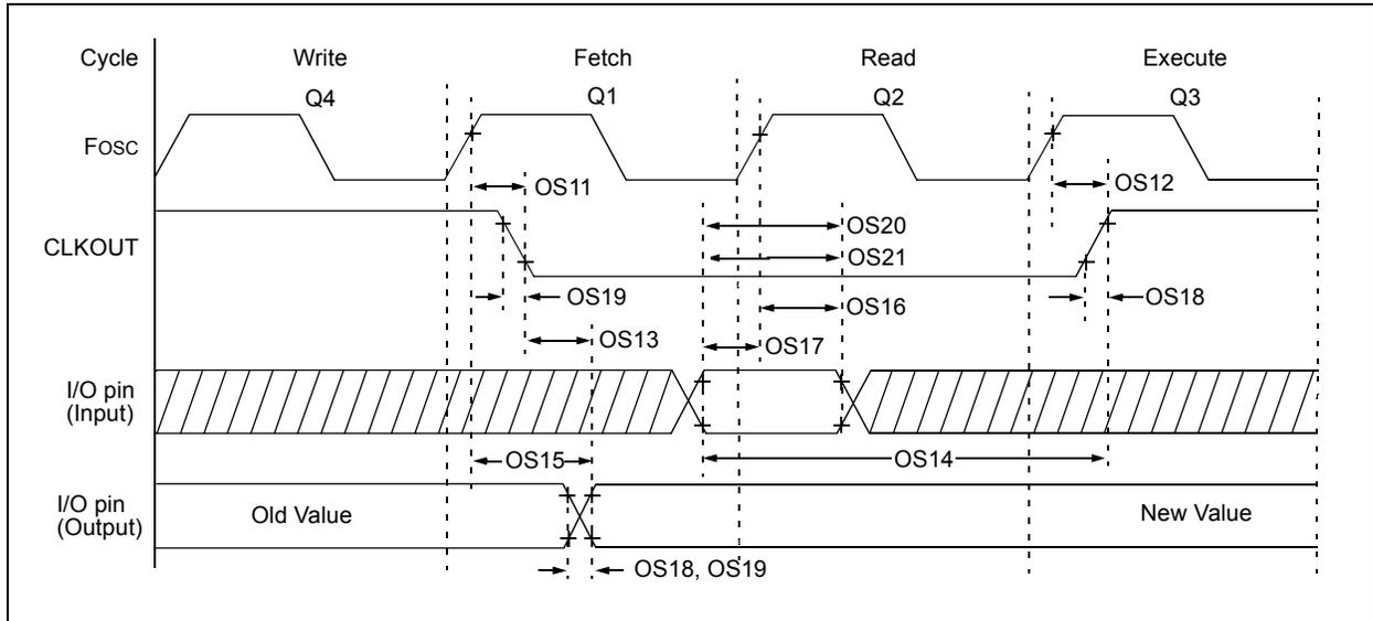
**TABLE 27-9: CLKOUT AND I/O TIMING PARAMETERS**
