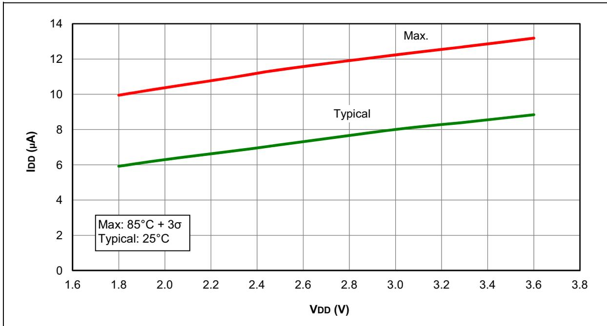
**FIGURE 28-2: I<sub>DD</sub>, EXTERNAL CLOCK (ECL), LOW-POWER MODE, F<sub>osc</sub> = 32 kHz, PIC12F1501 ONLY**
