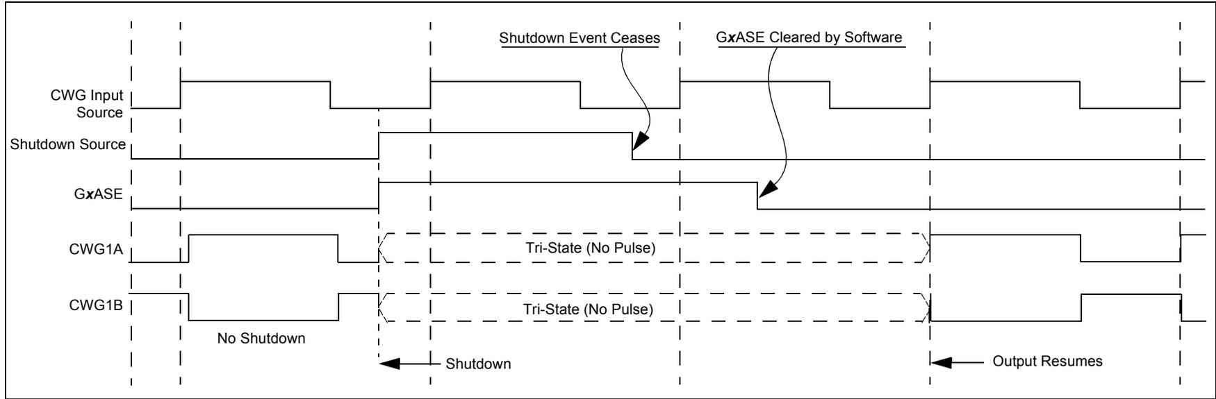
**FIGURE 24-6: SHUTDOWN FUNCTIONALITY, AUTO-RESTART ENABLED ( $GxARSEN = 1$ ,  $GxASDLA = 01$ ,  $GxASDLB = 01$ )**
