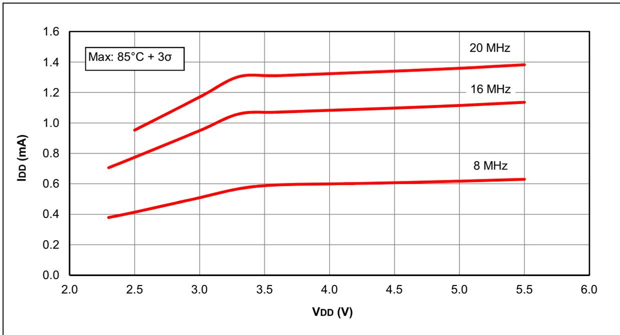
**FIGURE 28-13:  $I_{DD}$ , LFINTOSC,  $F_{osc} = 31$  kHz, PIC12LF1501 ONLY**
