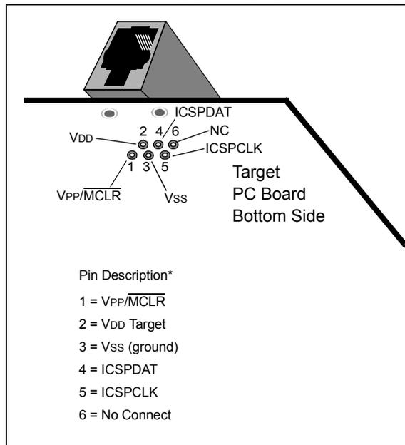
Another connector often found in use with the PICkit™ programmers is a standard 6-pin header with 0.1 inch spacing. Refer to [Figure 25-2](#).
