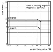
Lamp load (Inrush current: 6 times the rated current, Inrush current time: 2 cycles 5 Load current (A) Maximum switching frequency: 3 20 operations per minute 10 G9H-210S G9H-205S 1 20 40 60 Ambient temperature (°C)
