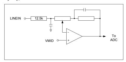
Figure 10 Line Input Schematic
