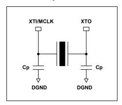
Figure 25 Crystal Oscillator Application Circuit
