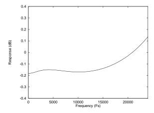
Figure 55 De-Emphasis Frequency Response (48kHz)
