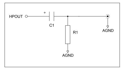
Figure 22 Headphone Output Application Drawing
