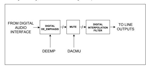
Figure 17 DAC Filter Schematic
