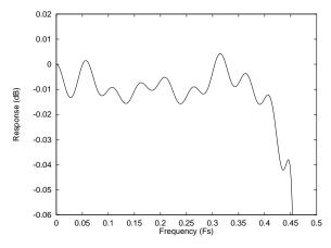
Figure 45 ADC Digital Filter Frequency Response -Type 1
