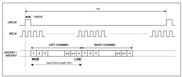
Figure 29 DSP/PCM Mode Audio Interface (mode A, LRP=1)
