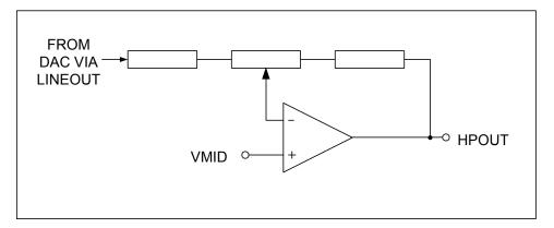
Figure 21 Headphone Amplifier Schematic
