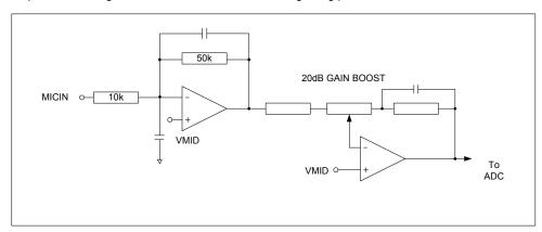
Figure 12 Microphone Input Schematic
