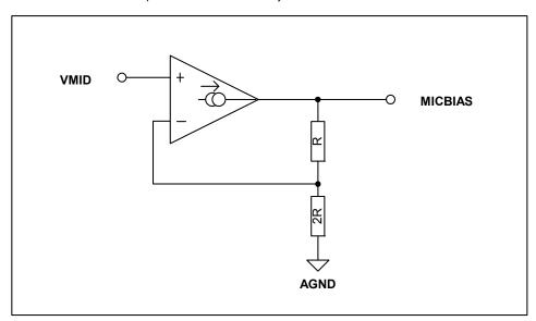
Figure 14 Microphone Bias Schematic
