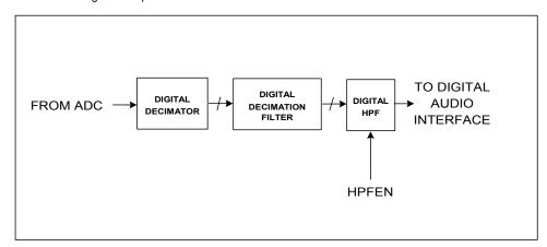
Figure 16 ADC Digital Filter
