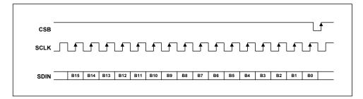
Figure 33 3-Wire Serial Interface
