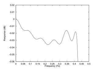
Figure 43 ADC Digital Filter Frequency Response -Type 0
