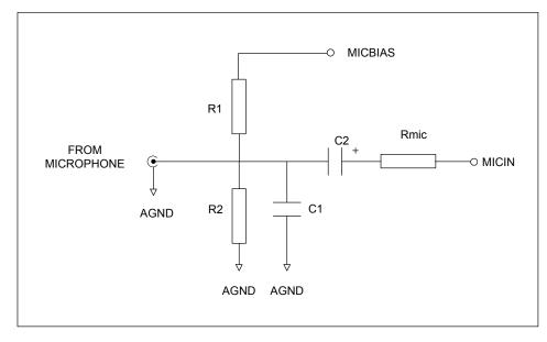
Figure 13 Microphone Input and Bias Application Drawing
