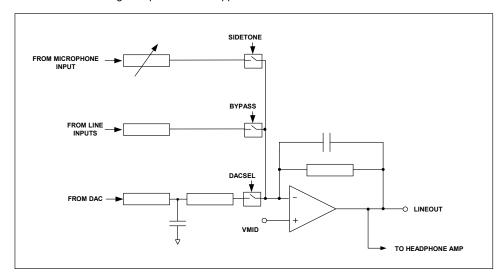
Figure 19 Line Output Schematic
