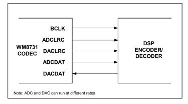
Figure 3 Master Mode Connection
