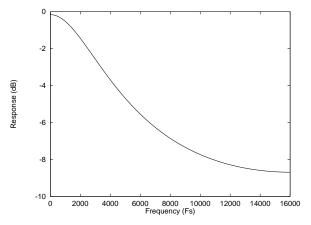
Figure 51 De-Emphasis Frequency Response (32kHz)
