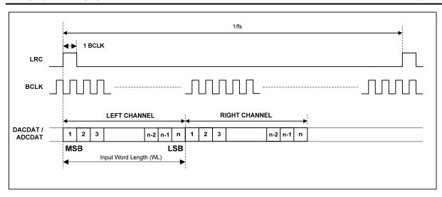
Figure 30 DSP/PCM Mode Audio Interface (mode B, LRP=0)
