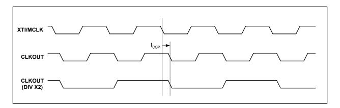
Figure 2 Clock Out Timing Requirements
