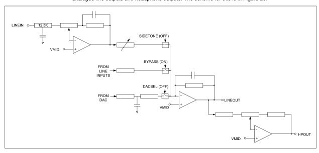
Figure 23 Signal Routing in Bypass Mode
