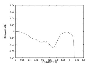
Figure 37 DAC Digital Filter Frequency Response -Type 1
