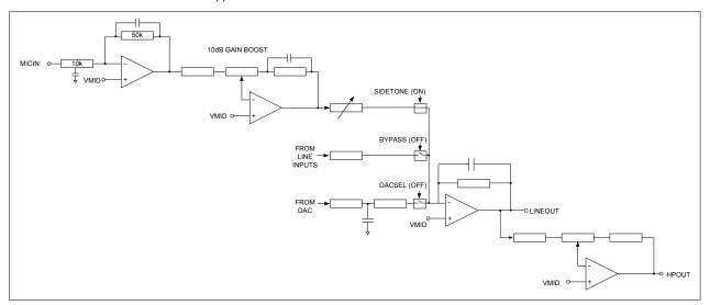
Figure 24 Side Tone Mode Schematic
