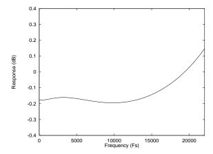
Figure 53 De-Emphasis Frequency Response (44.1kHz)
