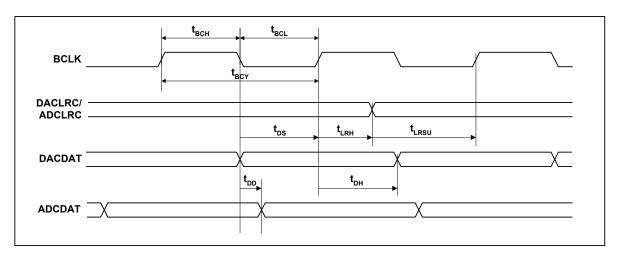
Figure 6 Digital Audio Data Timing - Slave Mode
