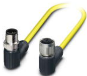
Sensor/actuator cable, 3-position, PVC, yellow, shielded, Plug angled M12 SPEEDCON, coding: A, on Socket angled M12 SPEEDCON, coding: A, cable length: 0.5 m
