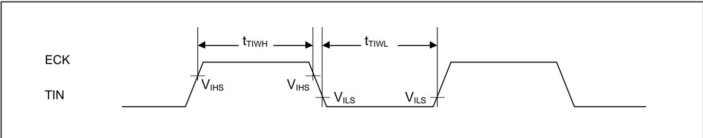
**Trigger input timing**
