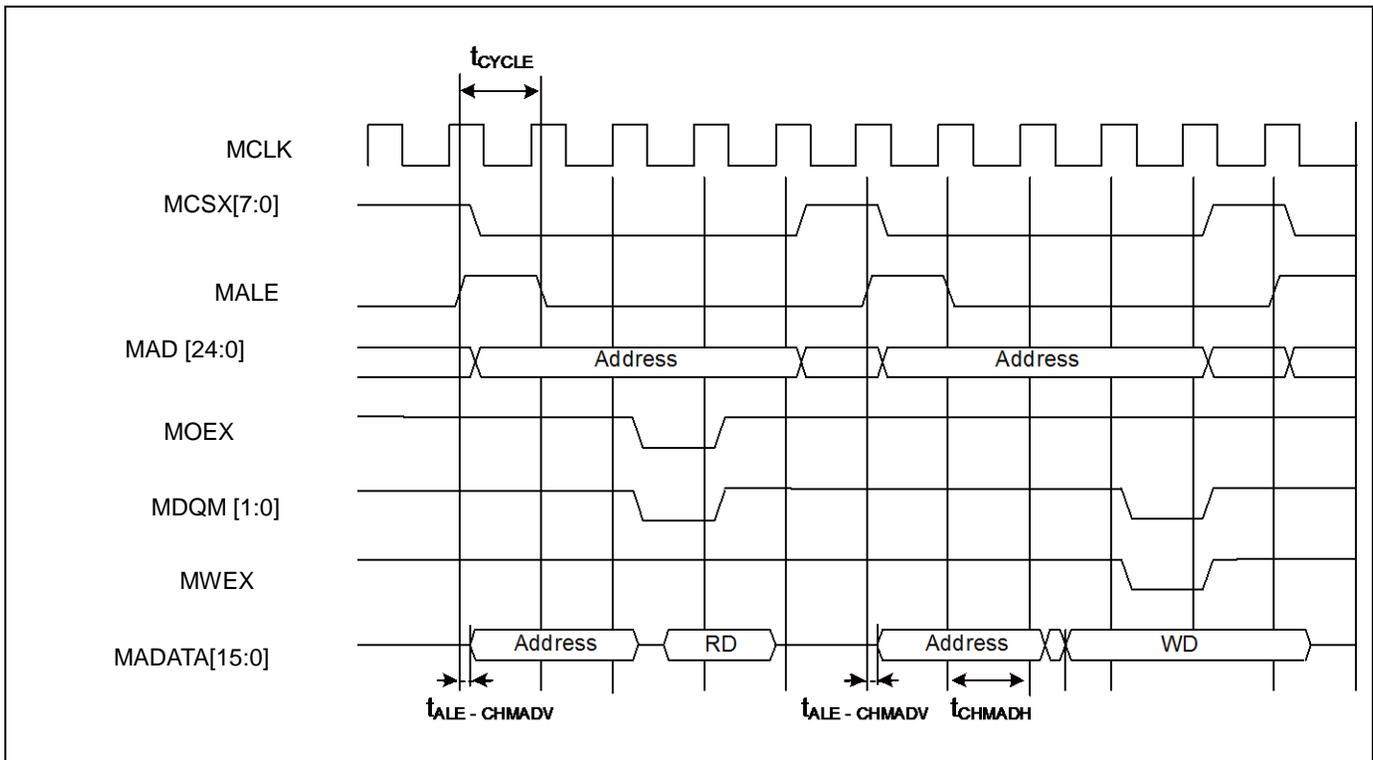
**Multiplexed Bus Access Synchronous SRAM Mode**
