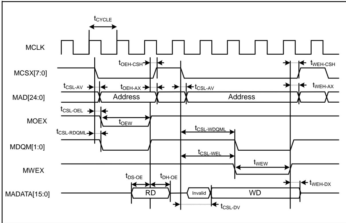
**Separate Bus Access Synchronous SRAM Mode**
