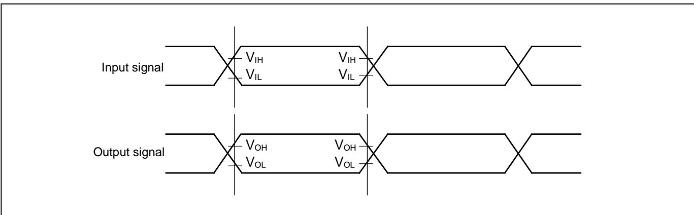
**Separate Bus Access Asynchronous SRAM Mode**
