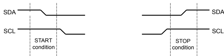
Figure 21-3. START and STOP Conditions
