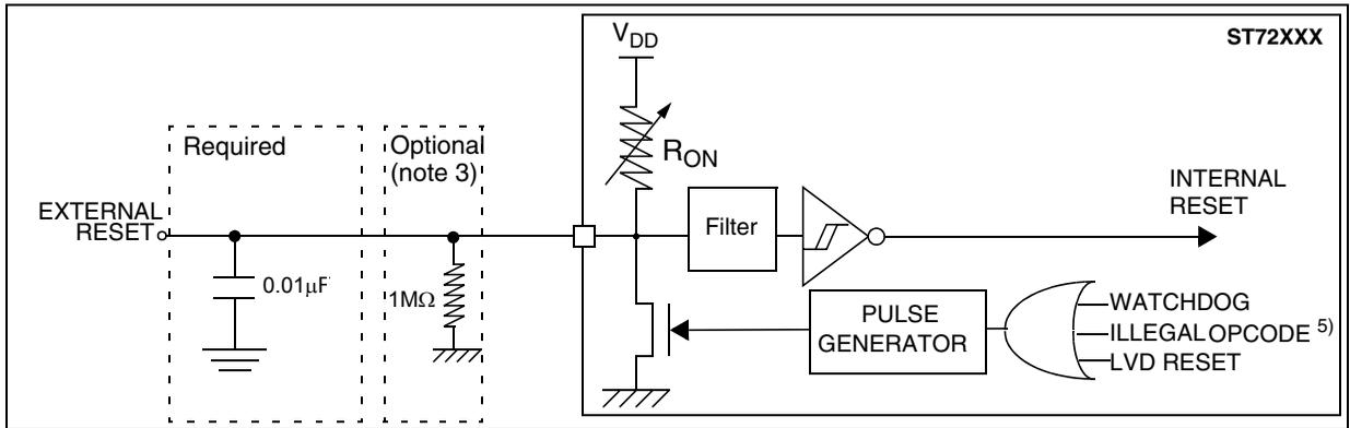
Figure 106.  $\overline{\text{RESET}}$  pin protection when LVD is disabled. <sup>1)</sup>
