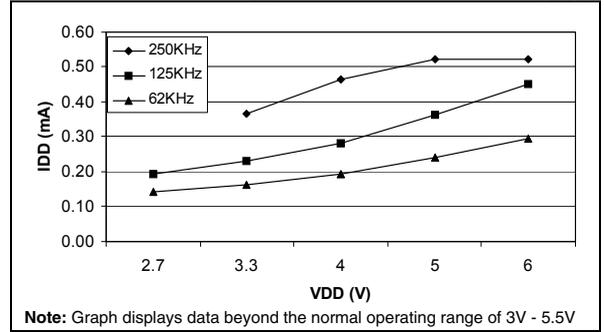
Figure 74. Typical  $I_{DD}$  in WAIT vs.  $f_{CPU}$
