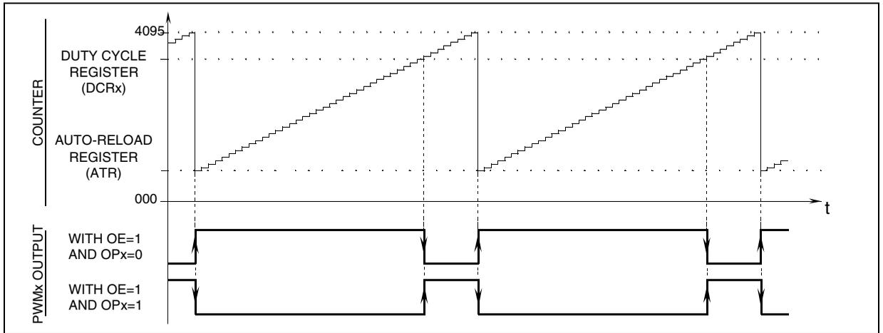
Figure 39. PWM Signal from 0% to 100% Duty Cycle
