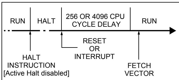
Figure 26. HALT Mode Flow-chart
