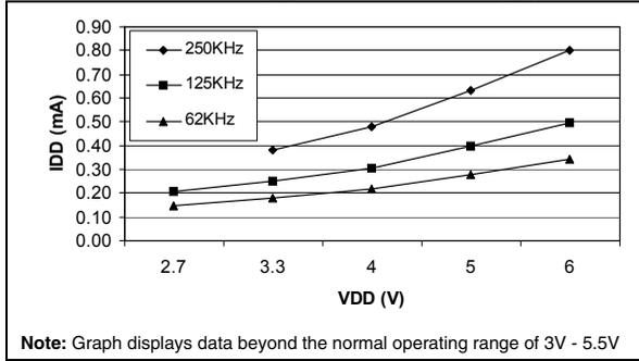
Figure 76. Typical  $I_{DD}$  in SLOW-WAIT vs.  $f_{CPU}$
