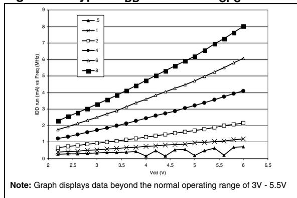
**Figure 72. Typical  $I_{DD}$  in RUN at  $f_{CPU} = 8\text{MHz}$**
