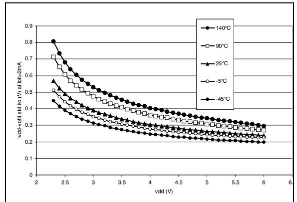
Figure 103. Typical  $V_{DD}-V_{OH}$  vs.  $V_{DD}$  (High Sink)
