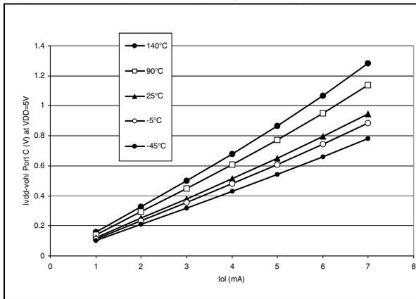
Figure 102. Typical  $V_{DD}-V_{OH}$  vs.  $V_{DD}$  (Standard)
