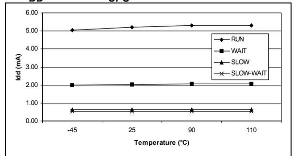
Figure 75. Typical  $I_{DD}$  in WAIT at  $f_{CPU} = 8MHz$
