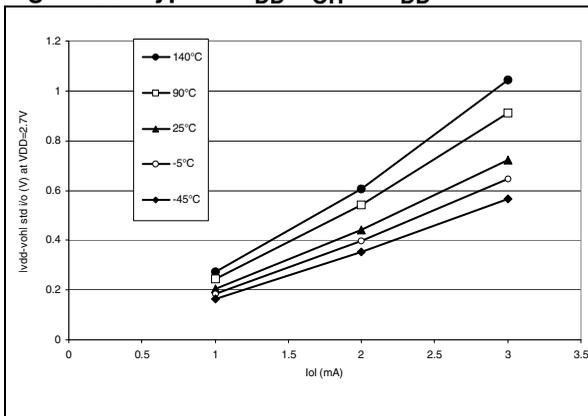
Figure 96. Typical  $V_{DD}-V_{OH}$  at  $V_{DD}=2.7V$  (HS)
