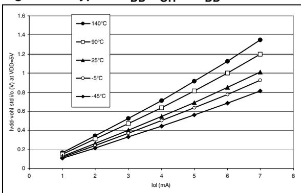
Figure 98. Typical  $V_{DD}-V_{OH}$  at  $V_{DD}=5V$  (HS)
