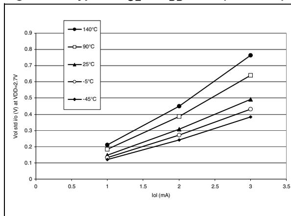
Figure 84. Typical  $V_{OL}$  at  $V_{DD}=2.7V$  (Port C)
