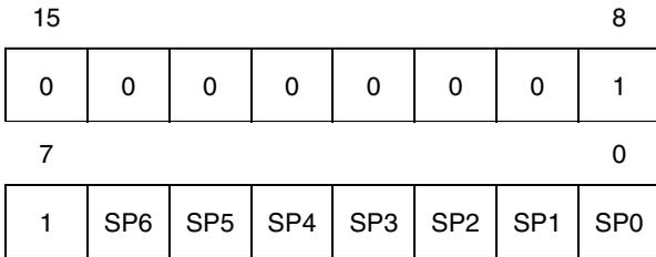
The Stack Pointer is a 16-bit register which is always pointing to the next free location in the stack. It is then decremented after data has been pushed onto the stack and incremented before data is popped from the stack (see Figure 12).
