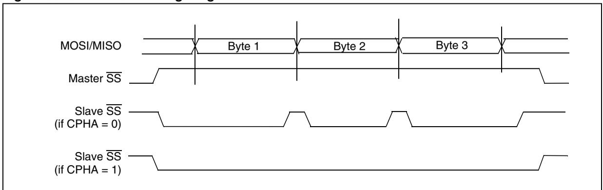
**Figure 56. Hardware/Software Slave Select Management**
