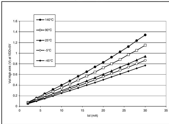
Figure 90. Typical  $V_{OL}$  vs.  $V_{DD}$  (standard I/Os)
