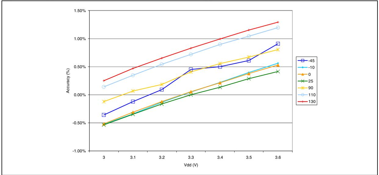
Figure 69. Typical RCCR1 vs V<sub>DD</sub> and Temperature
