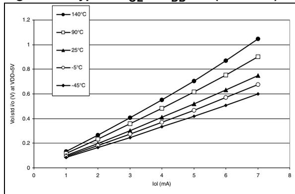
Figure 86. Typical  $V_{OL}$  at  $V_{DD}=5V$  (Port C)
