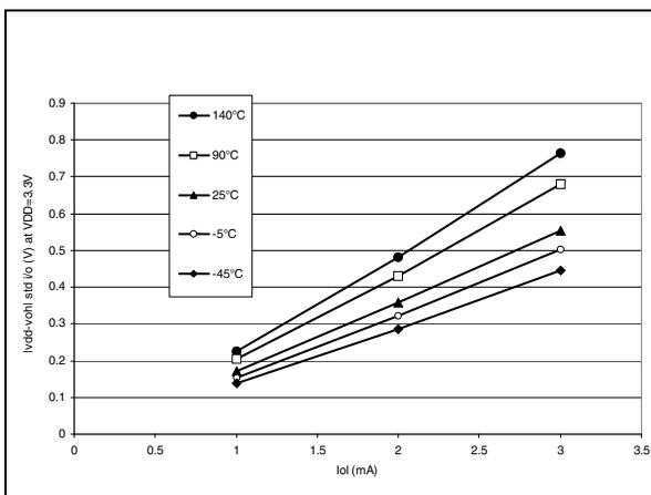
Figure 97. Typical  $V_{DD}-V_{OH}$  at  $V_{DD}=3.3V$  (HS)
