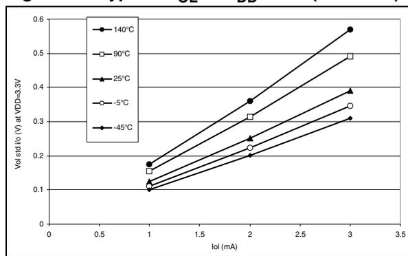
Figure 85. Typical  $V_{OL}$  at  $V_{DD}=3.3V$  (Port C)
