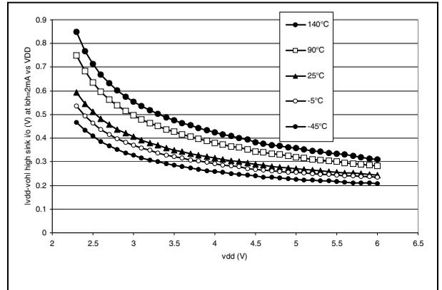
Figure 104. Typical  $V_{DD}-V_{OH}$  vs.  $V_{DD}$  (PORT C)
