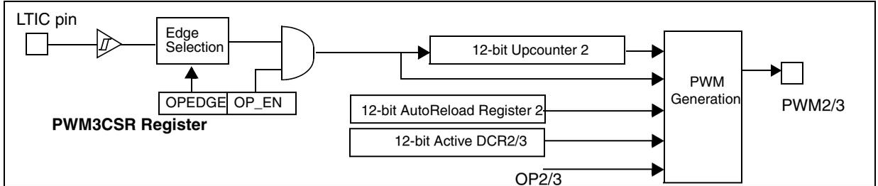
**Figure 48. One Pulse Mode and PWM Timing Diagram**
