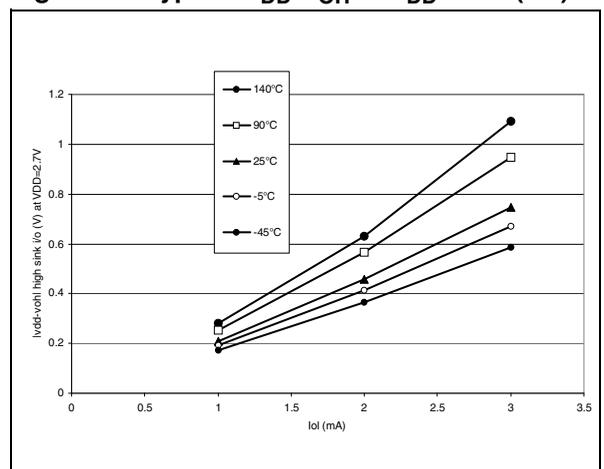
Figure 94. Typical  $V_{DD}-V_{OH}$  at  $V_{DD}=3.3V$
