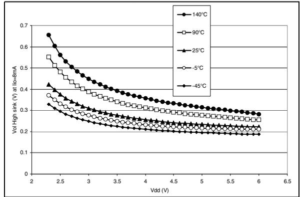
Figure 92. Typical  $V_{OL}$  vs  $V_{DD}$  (Port C)
