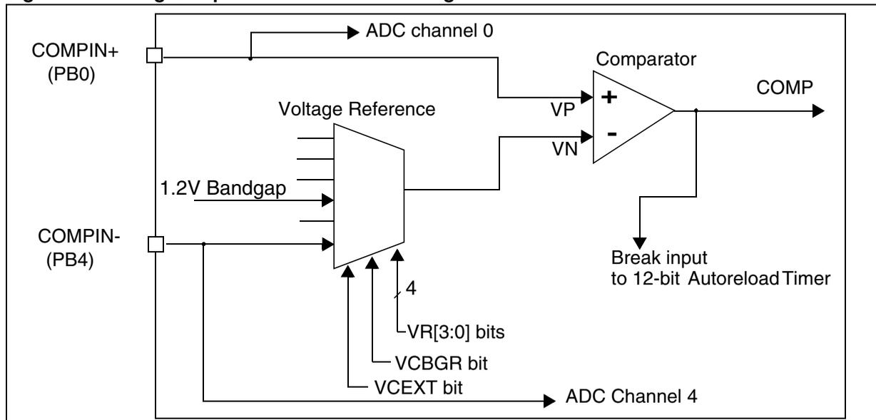
Figure 62. Analog Comparator
