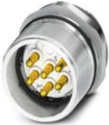
Device connector for front wall, straight, shielded: yes, SPEEDCON locking, M23, Number of positions: 8+1, Type of contact: Male connector, Solder connection, Seal, axial, Central fastening Pg13,5
