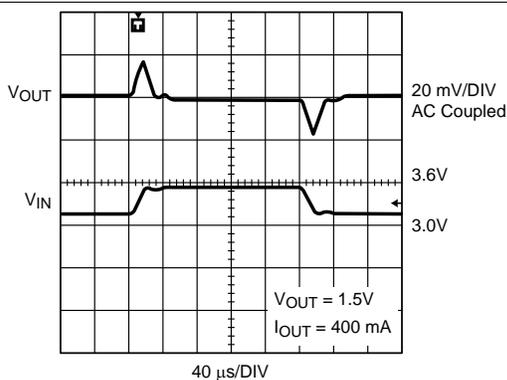
Figure 17. Line Transient Response (PWM Mode)
