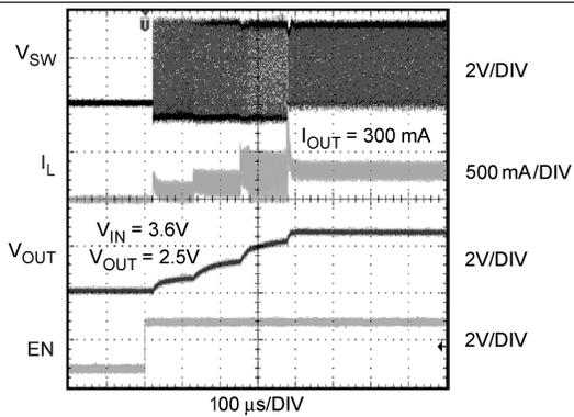
Figure 27. Start-Up into PWM Mode
