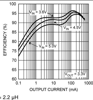
Figure 16. Efficiency vs Output Current
