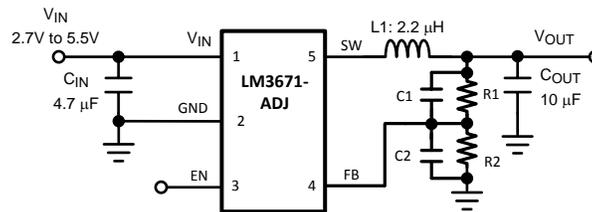
**Figure 35. Typical Application Circuit for ADJ Version**
