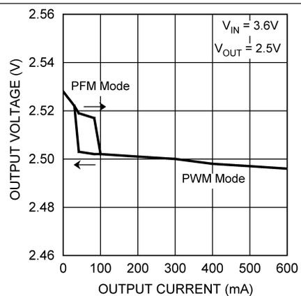
Figure 12. Output Voltage vs Output Current
