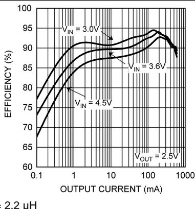
Figure 15. Efficiency vs Output Current
