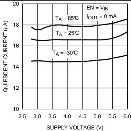
Figure 1. Quiescent Supply Current vs Supply Voltage
