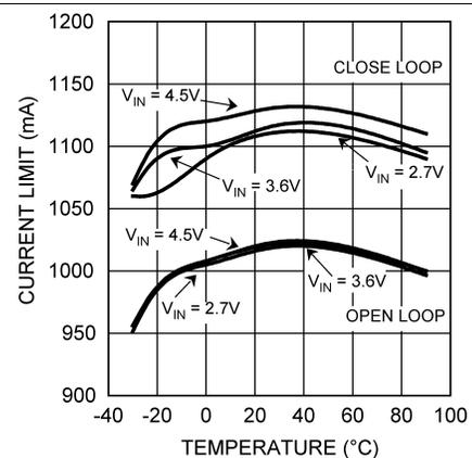
Figure 6. Open/Closed Loop Current Limit vs Temperature
