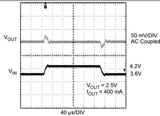
Figure 18. Line Transient Response (PWM Mode)
