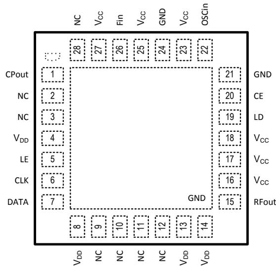
NOTE: Analog ground connected through exposed die attached pad.
