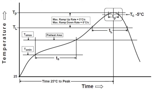
Soldering Iron condition: Soldering iron temperature 270°C±10°C.
