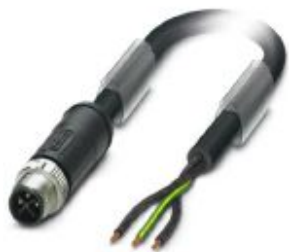
Power cable, 3-position, PVC, black, Plug straight M12, coding: S, on free cable end, cable length: 2 m, for AC current up to 16 A/230 V
