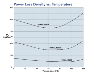
Measured on an 18/10/6mm toroid using the Clarke Hess 258 VAW at 100°C.
