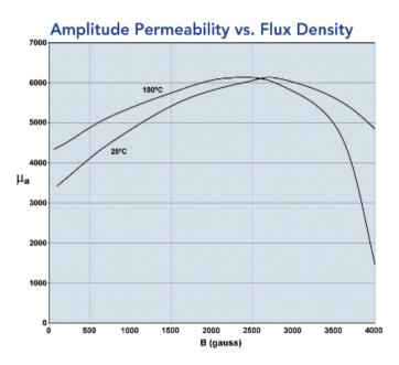
Measured on an 18/10/6mm toroid at 10kHz.
