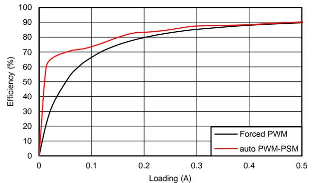
**Figure 7. 3.3-V Efficiency, Light Load**
