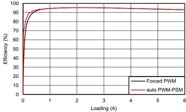
Figure 8. 5-V Efficiency
