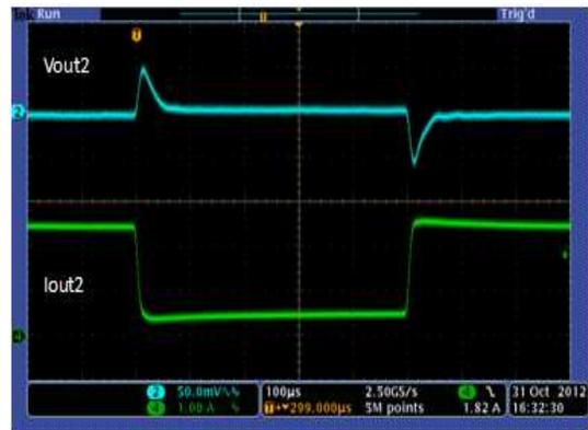
Figure 25. Load Transient, Buck 2 (0.5 A - 2.5 A)
