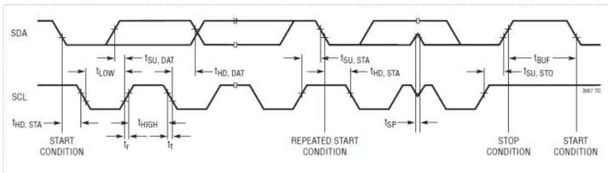
**Figure 37. I<sup>2</sup>C Interface Timing Diagram**
