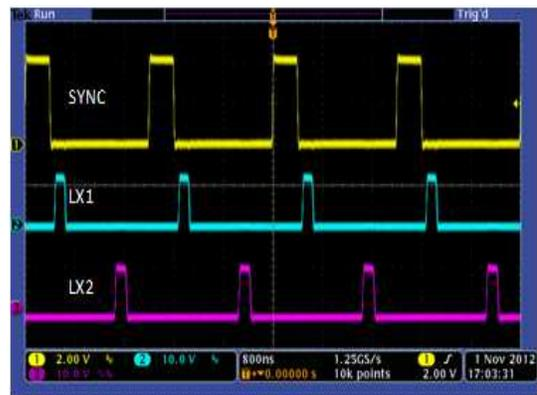
Figure 31. Synchronization at 500 kHz
