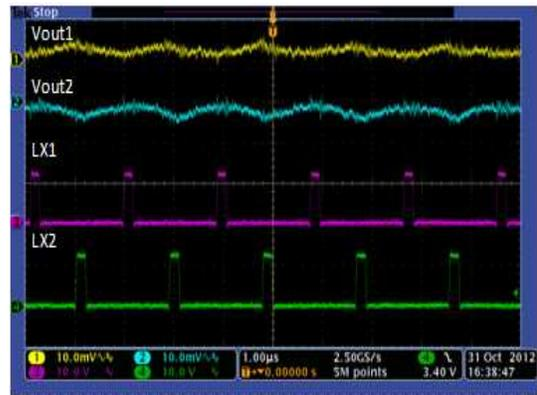
**Figure 19. Output Ripple at 3.5 A, Forced PWM**
