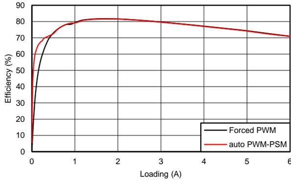
**Figure 2. 0.8-V Efficiency**
