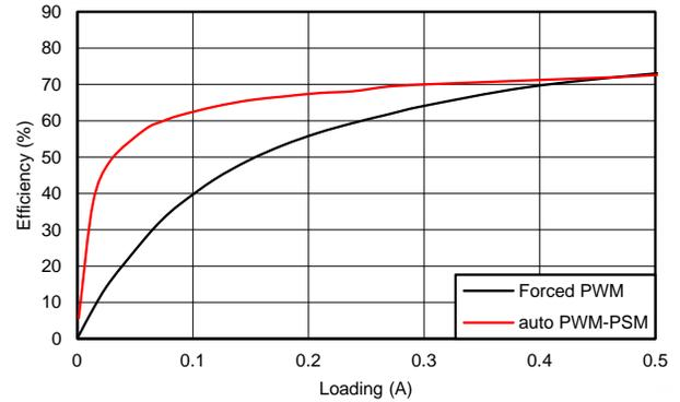
**Figure 3. 0.8-V Efficiency, Light Load**
