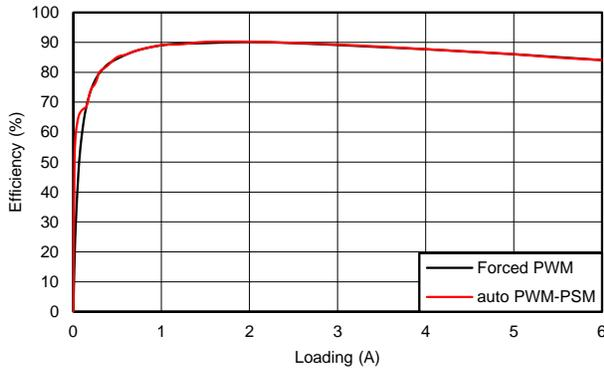
**Figure 4. 1.8-V Efficiency**
