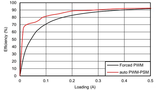
Figure 9. 5-V Efficiency, Light Load
