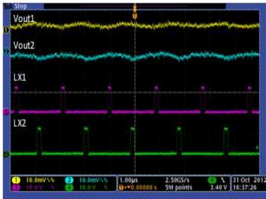
**Figure 18. Output Ripple at 0 A, Forced PWM**
