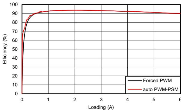
**Figure 6. 3.3-V Efficiency**
