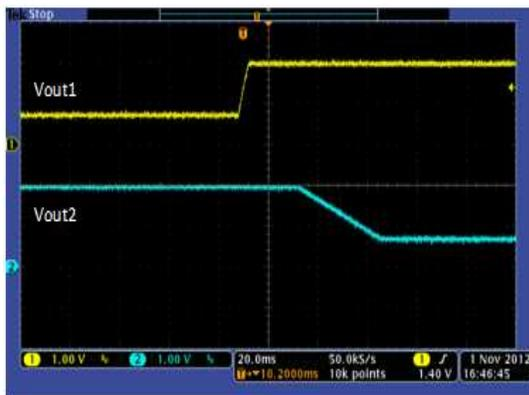
Figure 30. Voltage Change With I<sup>2</sup>C Control
