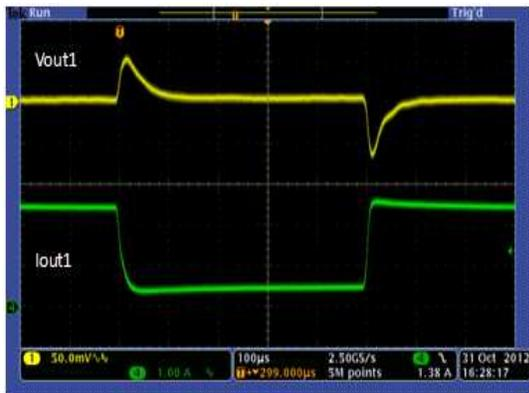
Figure 24. Load Transient, Buck 1 (0.5 A - 2.5 A)
