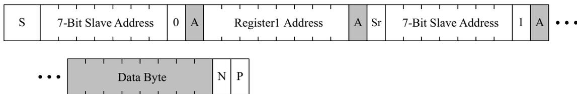
Figure 39. I<sup>2</sup>C Read Data Format
