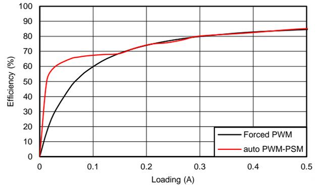
**Figure 5. 1.8-V Efficiency, Light Load**
