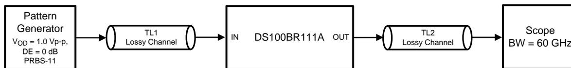
Figure 11. Test Setup Connections Diagram
