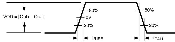
**Figure 1. Output Rise and Fall Transition Times**
