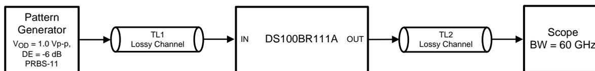
Figure 12. Test Setup Connections Diagram
