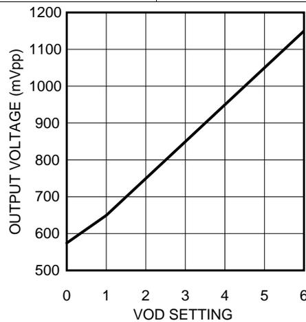
Figure 7. Output Voltage vs. Output Voltage Setting
