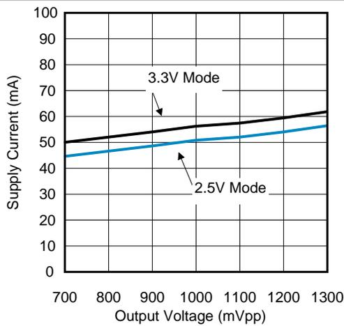
Figure 5. Supply Current vs. Output Voltage Setting
