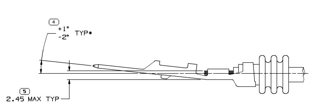
TERMINAL, SEAL AND CABLE ALIGNMENT SCALE 5:1
