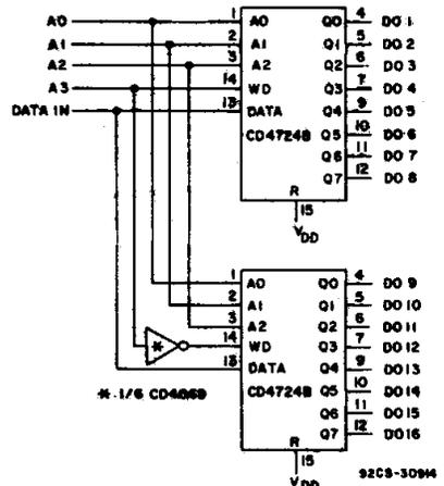
Fig. 14— 1 of 16 decoder/demultiplexer.
