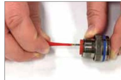
Note: All plastic tools are double-ended. The colored side is the insertion tool and the white side is the removal tool.
