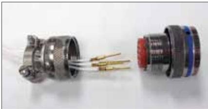
2. Use proper plastic or metal insertion tool for corresponding contact. (Consult tool table on preceding page). Slide correct tool (with plastic tool use colored end) over wire insulation and slide forward until tool bottoms against rear contact shoulder.
