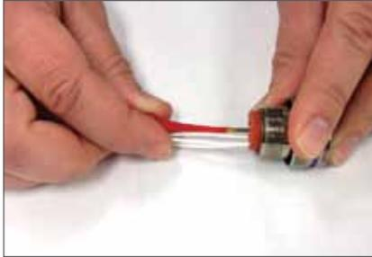
5. After all contacts are inserted, fill any empty cavities with wire sealing plugs. (Refer to sealing plug charts for Series III on page 18, for Series I, II, and SJT on page 19.)
