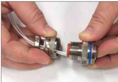
2. Use proper plastic or metal removal tool for corresponding contact. (Consult tool table on page 277). Slide correct size tool over wire insulation.
