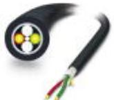
Highly rugged PCF round cable (IP20 heads only) for assembly and for outdoor installation with integrated moisture barrier as well as rodent-proof scrim. Individual elements made from highly flexible FRNC material. The wire is ozone and UV resistant with a very rugged polyethylene outer sheath.
