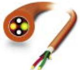
rugged PCF installation cable for inner areas with highly tear-proof aramid strain-relief elements. Individual elements made from highly flexible FRNC material. The cable is halogen-free, ozone and UV resistant and has a rugged polyurethane (PUR) outer sheath.
