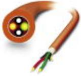
rugged PCF installation cable (IP20 heads only) for inner areas with highly tear-proof aramid strain-relief elements. Individual elements made from highly flexible FRNC material. The cable is halogen-free, ozone and UV resistant and has a rugged polyurethane (PUR) outer sheath.
