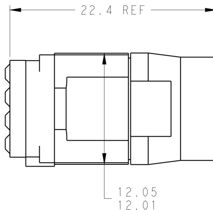
△<sub>1</sub> FRONT & REAR INSULATORS: HIGH-TEMP THERMOPLASTIC OR THERMOSET EPOXY PER ASTM D5948. CONTACT RETENTION CLIPS: STAINLESS STEEL PER AISI 302 OR COPPER ALLOY PER ASTM B194, REAR GROMMET & INTERFACIAL SEAL: FLUOROSILICONE ELASTOMER PER MIL-R-25988 B EXCEPT 4.6.6.1.
