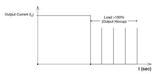
It is not recommended to prolong the duration of I<sub>O</sub> when it is <150% but >100%, since it may cause damage to the PSU.
