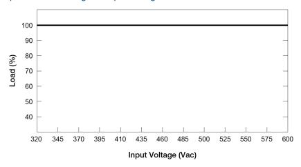
No output power de-rating across the entire input voltage range 3 x 320-600Vac (3-Phase) or 2 x 360-600Vac (2-Phase)
