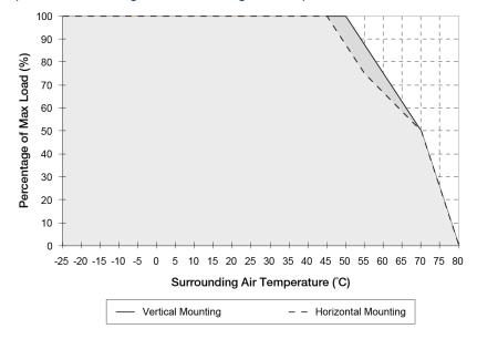
Fig. 1 De-rating for Vertical Mounting Orientation
