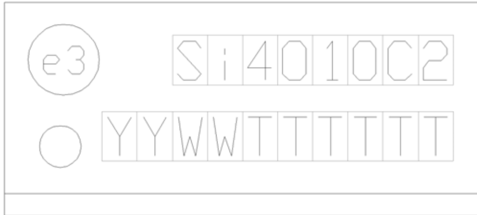
Figure 1. Si4010 Top Marking
