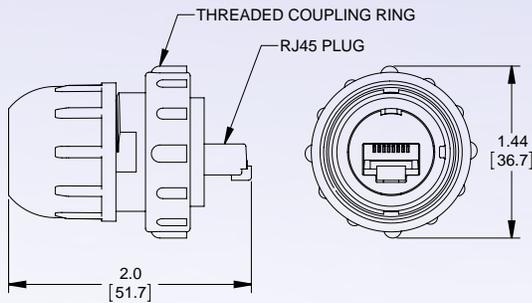
**RJ45 FIELD INSTALLABLE CABLE PLUG ASSEMBLY (QUICK CONNECT COUPLING)**
