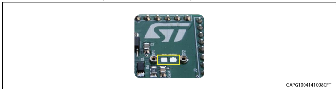
Figure 5: Pads for soldering SMD resistor
