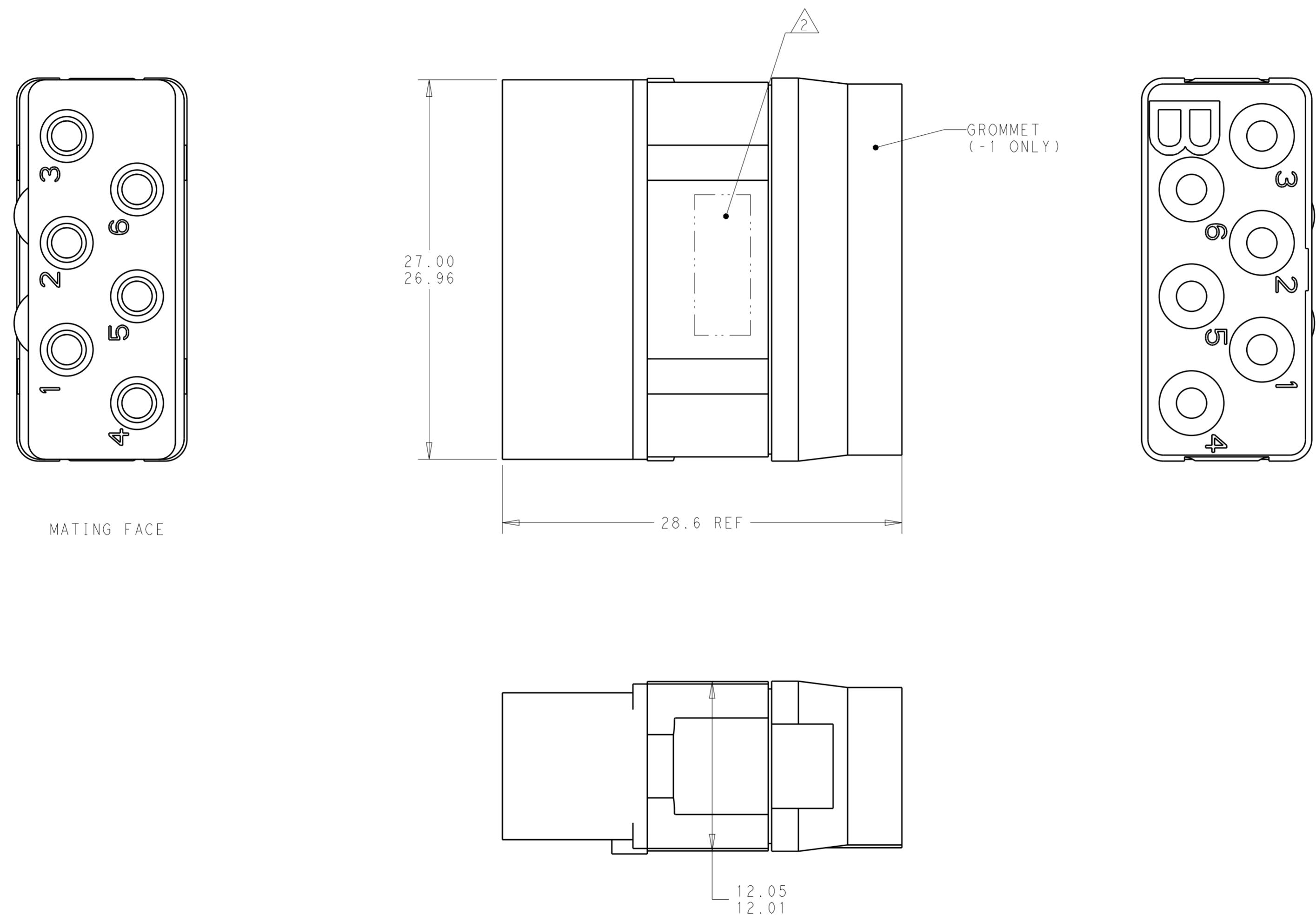
△1 FRONT & REAR INSULATOR: HIGH-TEMP THERMOPLASTIC OR THERMOSET EPOXY PER ASTM D5948.
