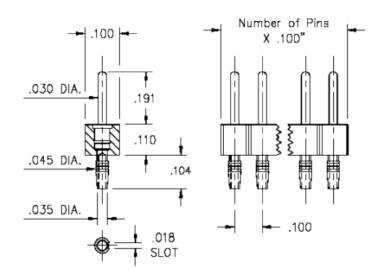
**Description:** Interconnect Header Solderless Press-Fit Pin Header .030" (0,76mm) Pin Head Single Row Through Hole Plating Code: 10 Shell Plating: 10  $\mu$ " Gold over 100  $\mu$ " Nickel
