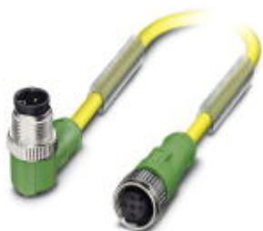
Sensor/actuator cable, 4-position, PUR/PVC, yellow, Plug angled M12, A-coded, on Socket straight M12, A-coded, cable length: 3 m, DESINA
