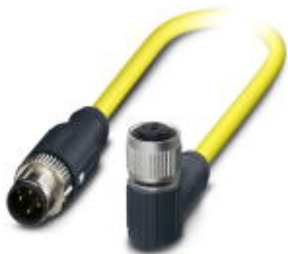
Sensor/actuator cable, 4-position, PVC, yellow, shielded, Plug straight M12 SPEEDCON, coding: A, on Socket angled M12 SPEEDCON, coding: A, cable length: 1.5 m
