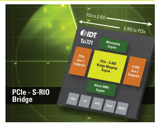
IDT is the industry's leading supplier of RapidIO<sup>®</sup> and PCI Express<sup>®</sup> Interconnect solutions, providing a broad portfolio of switches, bridges, IP and development platforms for defense, aerospace, video, imaging and wireless markets. The Tsi721 is IDT's solution for hardware based PCIe Gen 2 to RapidIO Gen 2 protocol conversion in a bridging device
