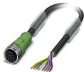
Sensor/actuator cable, 8-position, PUR halogen-free, black-gray RAL 7021, free cable end, on Socket straight M12, A-coded, cable length: 2 m
