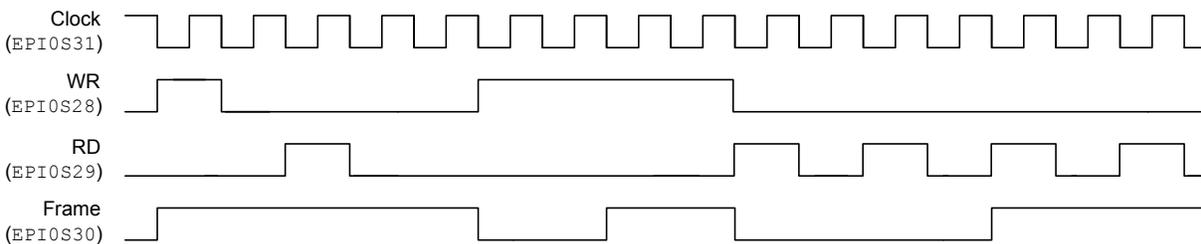
When `FRMCNT=2`, the FRAME signal transitions the rising edge of the WR or RD strobes for every third access, and so on for every value of `FRMCNT`, see Figure 9-21 on page 475.
