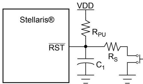
Typical  $R_{PU} = 10 \text{ k}\Omega$
