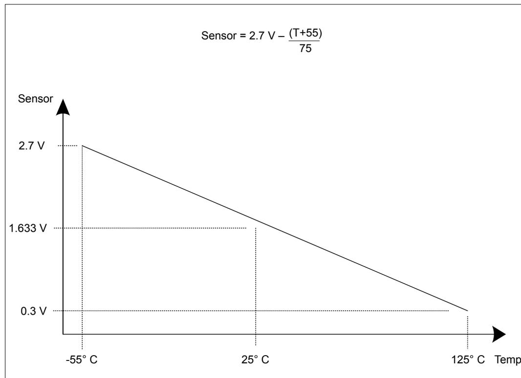
The temperature sensor reading can be sampled in a sample sequence by setting the *TSn* bit in the *ADCSSCTLn* register. The temperature reading from the temperature sensor can also be given as a function of the ADC value. The following formula calculates temperature (in °C) based on the ADC reading:
