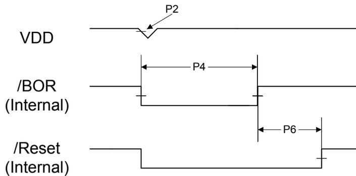
Figure 25-6. Power-On Reset and Voltage Parameters
