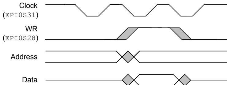
**Figure 9-24. EPI Clock Operation, CLKGATE=1, WR2CYC=1**
