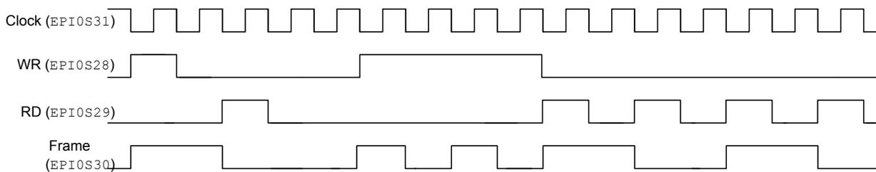
When `FRMCNT=1`, the FRAME signal transitions on the rising edge of the WR or RD strobes for every other access, see Figure 9-20 on page 475.
