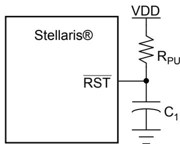
$R_{\text{PU}} = 1$  k $\Omega$  to 100 k $\Omega$
