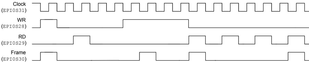
When `FRM50` is set, the FRAME signal transitions on the rising edge of either the WR or RD strobes. When `FRMCNT=0`, the FRAME signal transitions on the rising edge of WR or RD for every access, see Figure 9-19 on page 475.
