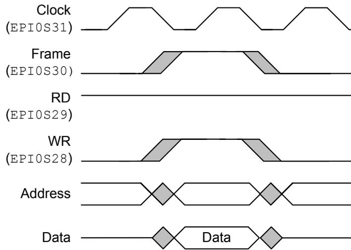
**Figure 9-14. Two-Cycle Read, Write Accesses, FRM50=0, FRMCNT=0, RDCYC=1, WRCYC=1**
