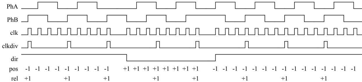
The period of the timer is configurable by specifying the load value for the timer in the **QEI Timer Load (QEILOAD)** register. When the timer reaches zero, an interrupt can be triggered, and the hardware reloads the timer with the **QEILOAD** value and continues to count down. At lower encoder speeds, a longer timer period is required to be able to capture enough edges to have a meaningful result. At higher encoder speeds, both a shorter timer period and/or the velocity predivider can be used.
