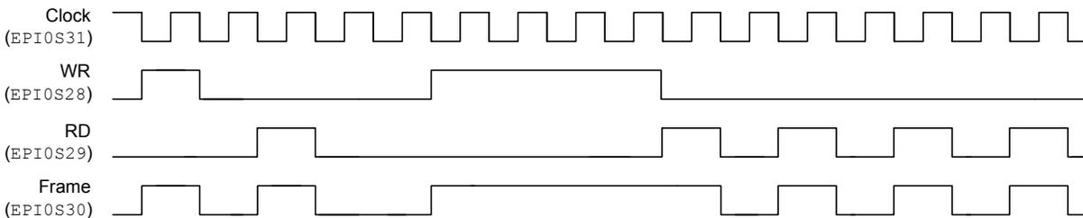
If the FRMCNT field is 0x1, then the FRAME signal pulses high during every other read or write access, see Figure 9-17 on page 474.
