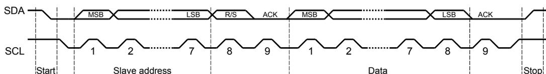
The first seven bits of the first byte make up the slave address (see Figure 15-5). The eighth bit determines the direction of the message. A zero in the R/S position of the first byte means that the master transmits (sends) data to the selected slave, and a one in this position means that the master receives data from the slave.
