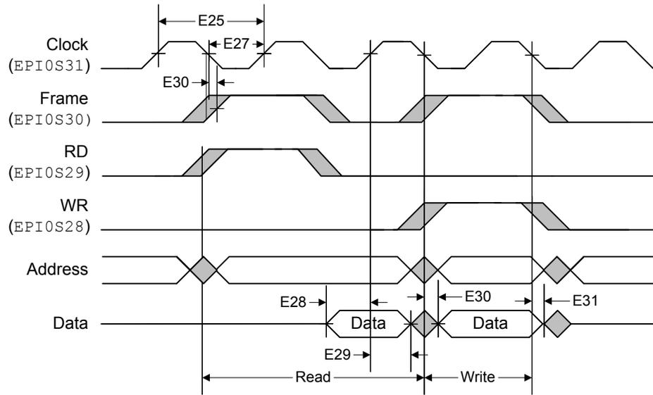
The above figure illustrates accesses where the FRM50 bit is clear, the FRMCNT field is 0x0, the RD2CYC bit is clear, and the WR2CYC bit is clear.
