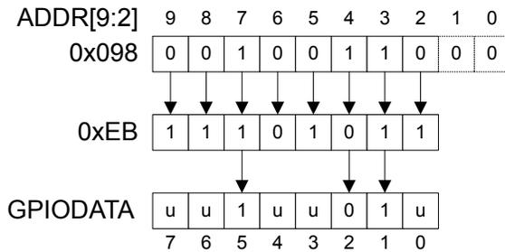
During a read, if the address bit associated with the data bit is set, the value is read. If the address bit associated with the data bit is cleared, the data bit is read as a zero, regardless of its actual value. For example, reading address GPIODATA + 0x0C4 yields as shown in Figure 8-4.
