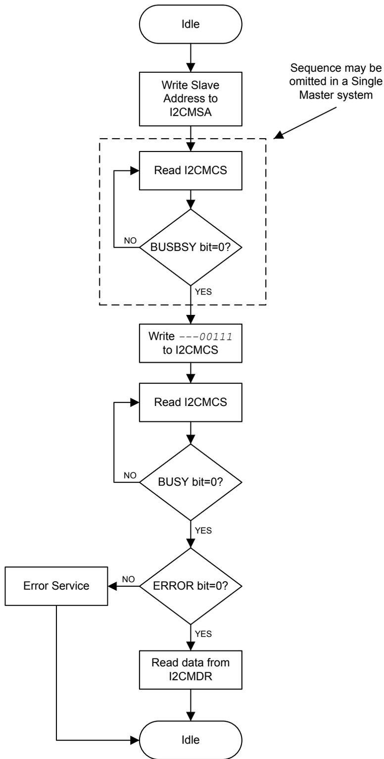
Figure 15-9. Master TRANSMIT with Repeated START
