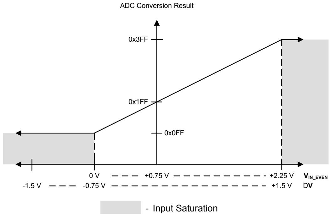
Figure 12-11. Differential Sampling Range,  $V_{IN\_ODD} = 2.25\text{ V}$
