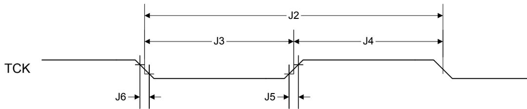
Figure 25-9. JTAG Test Access Port (TAP) Timing
