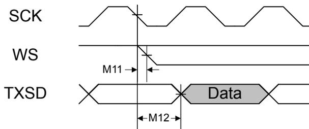
Figure 25-29. I<sup>2</sup>S Master Mode Receive Timing
