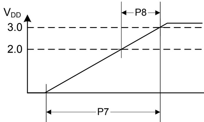
Figure 25-7. Voltage Requirements When Using an External  $V_{DDC}$  Source
