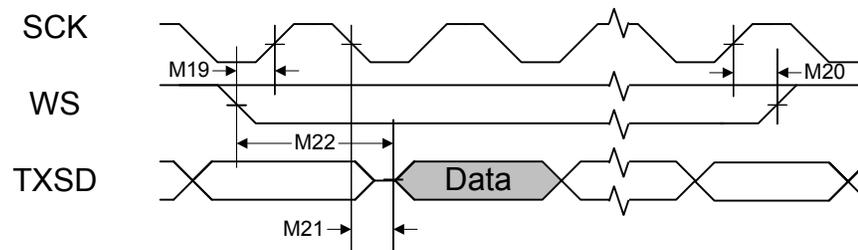
Figure 25-31. I<sup>2</sup>S Slave Mode Receive Timing
