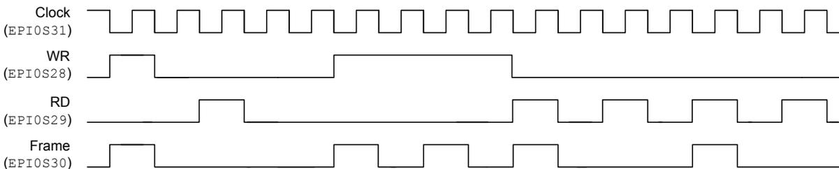
If the FRMCNT field is 0x2 and FRM50 is clear, then the FRAME signal pulses high during every third access, and so on for every value of FRMCNT, see Figure 9-18 on page 475.
