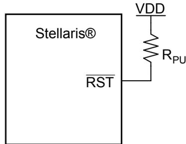
$R_{\text{PU}} = 0$  to 100 k $\Omega$
