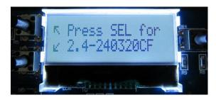
11. When prompted, press the SEL button to continue the demonstration program and scroll through the corresponding files on the SD Card. See Appendix B for SD Card file formatting and editing. You may see a blink on the display as the SD Card is being read and the display is being re-initialized and written.
