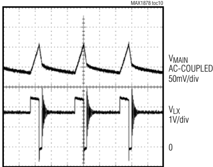
STEP-DOWN LIGHT-LOAD SWITCHING WAVEFORMS
