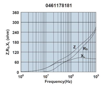
Impedance, reactance, and resistance vs. frequency.
