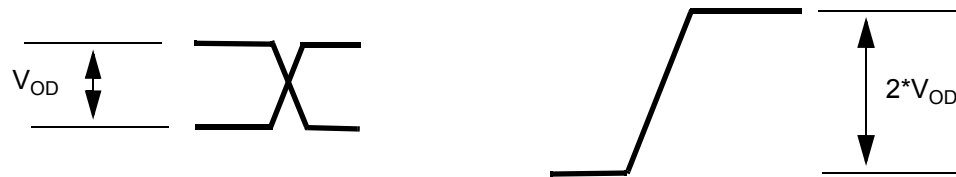
Figure 20 - Differential Voltage Parameter
