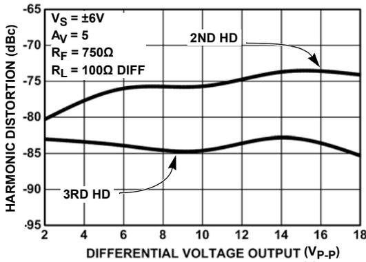
FIGURE 10. HARMONIC DISTORTION AT 3MHZ
