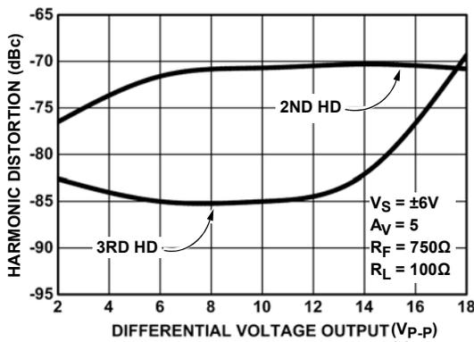
FIGURE 12. HARMONIC DISTORTION AT 5MHZ
