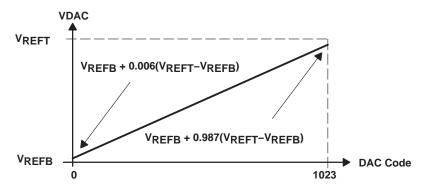
Figure 40. Clamp DAC Output Voltage Versus DAC Register Code Value
