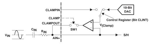
Figure 38. Schematic of Clamp Circuitry
