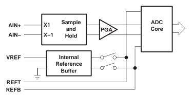
Figure 26. ADC Reference Generation, MODE = AGND
