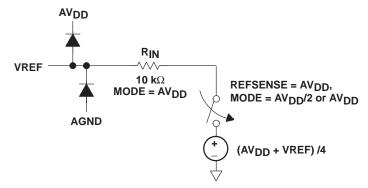
Figure 45. Equivalent Circuit of VREF
