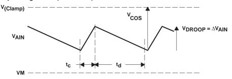
Figure 47. Approximate Waveforms at AIN During Droop and Clamping
