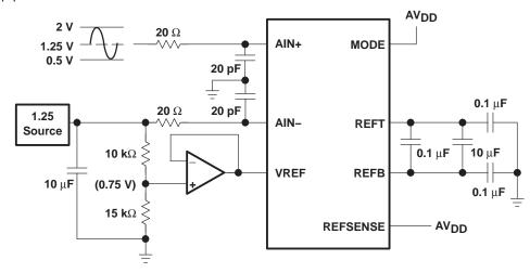
Figure 36. Operating Configuration: 1.5-V Single-Ended Input, External VREF Source
