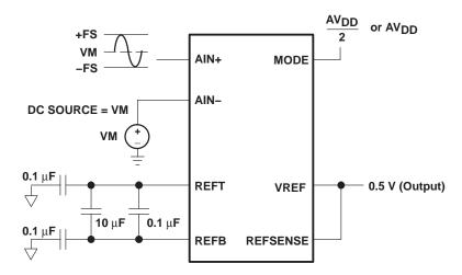
Figure 29. Internal Reference Mode, 0.5-V Reference Span, Single-Ended Input
