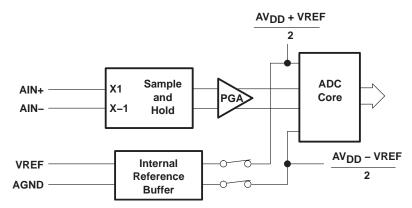
Figure 27. ADC Reference Generation, MODE = AV<sub>DD</sub>/2
