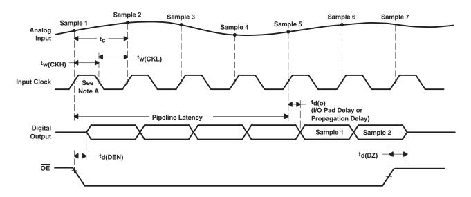
NOTE A: All timing measurements are based on 50% of edge transition.
