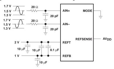
Figure 37. Operating Configuration: 0.8-V Differential Input and External ADC References clamp operation
