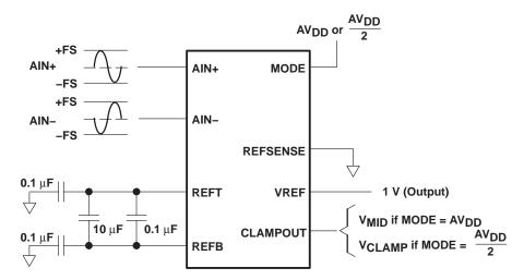
Figure 28. Internal Reference Mode, 1-V Reference Span
