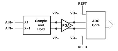
Figure 25. Analog Input Signal Flow
