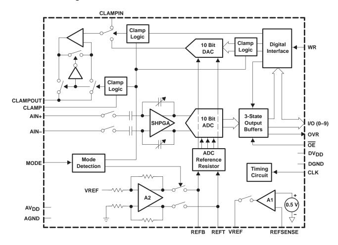
NOTE: A1 – Internal bandgap reference A2 – Internal ADC reference generator
