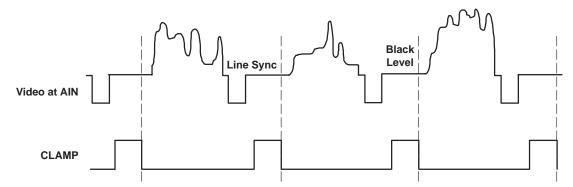
Figure 39. Example Waveforms for Line-Clamping to a Video Input Black Level
