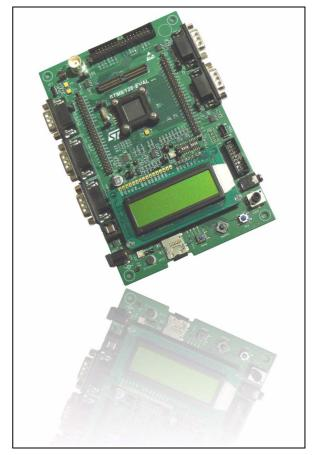
The full range of hardware features helps you to evaluate all peripherals (including motor control, CAN, micro SD Card, smartcard, UART, LIN, IrDA) and develop your own applications. Extension headers make it possible to easily connect a daughterboard or wrapping board for your specific application.
