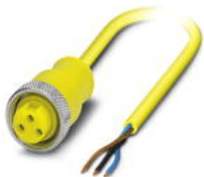
Sensor/actuator cable, 3-position, PVC, yellow, free cable end, on Socket straight 7/8"-16UNF, A-coded, cable length: 2 m
