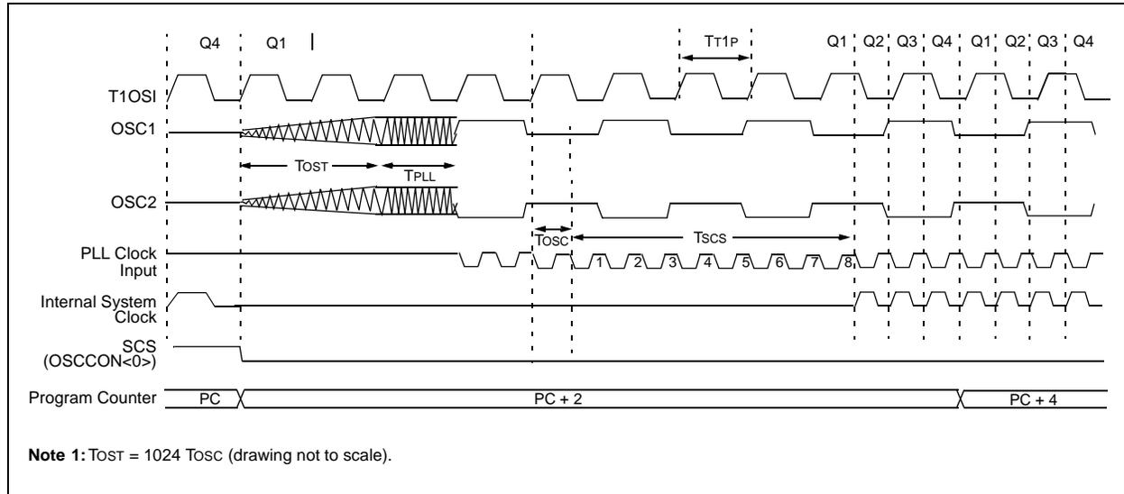
If the main oscillator is configured in the RC, RCIO, EC or ECIO modes, there is no oscillator start-up time-out. Operation will resume after eight cycles of the main oscillator have been counted. A timing diagram,
