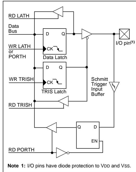
**FIGURE 10-18: RH7:RH4 PINS BLOCK DIAGRAM IN I/O MODE**
