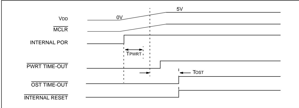
**FIGURE 3-7: TIME-OUT SEQUENCE ON POR W/PLL ENABLED ( $\overline{\text{MCLR}}$  TIED TO  $V_{\text{DD}}$  VIA 1 k $\Omega$  RESISTOR)**
