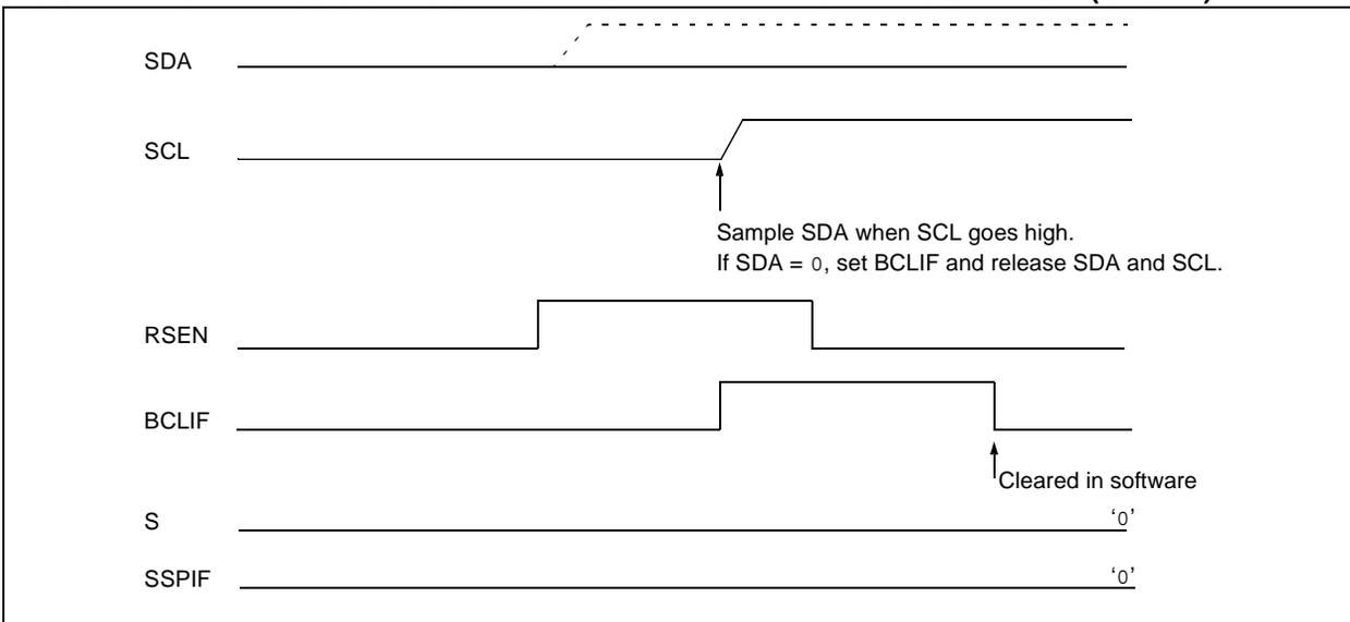
**FIGURE 17-30: BUS COLLISION DURING REPEATED START CONDITION (CASE 2)**
