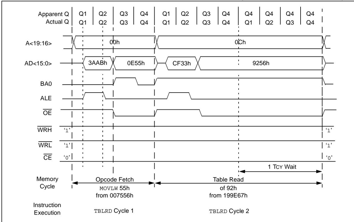
**FIGURE 6-5: EXTERNAL MEMORY BUS TIMING FOR TBLRD (EXTENDED MICROCONTROLLER MODE)**
