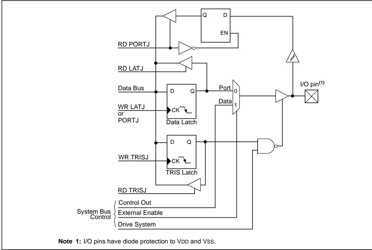
**FIGURE 10-22: RJ7:RJ6 PINS BLOCK DIAGRAM IN SYSTEM BUS MODE**
