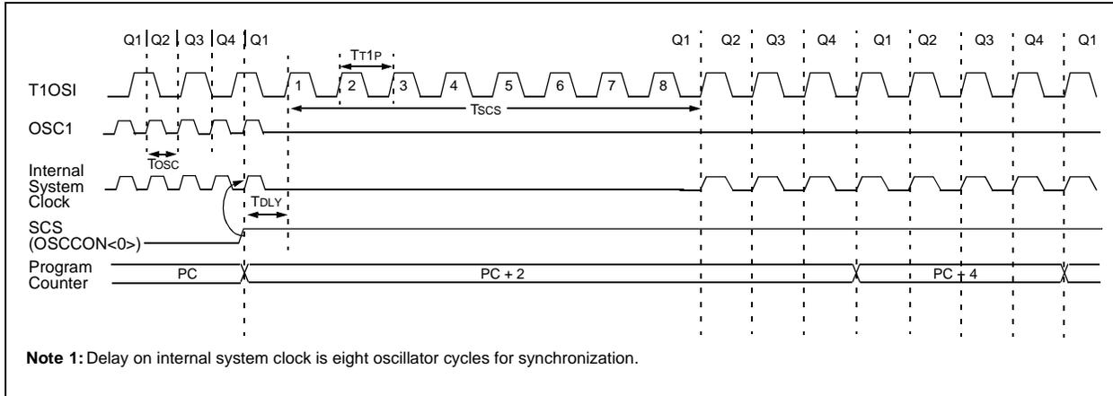
The sequence of events that takes place when switching from the Timer1 oscillator to the main oscillator will depend on the mode of the main oscillator. In addition to eight clock cycles of the main oscillator, additional delays may take place.
