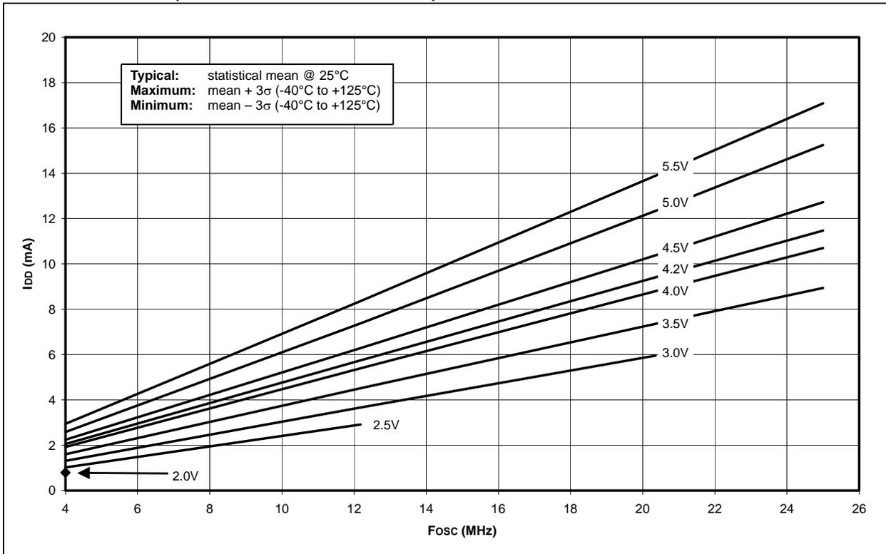
**FIGURE 27-22: TYPICAL I<sub>DD</sub> vs. F<sub>osc</sub> OVER V<sub>DD</sub> (HS/PLL MODE) (PIC18F8520 DEVICES ONLY)**
