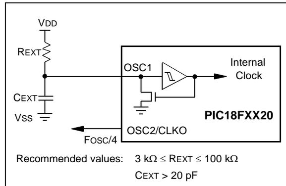
The RCIO Oscillator mode functions like the RC mode, except that the OSC2 pin becomes an additional general purpose I/O pin. The I/O pin becomes bit 6 of PORTA (RA6).
