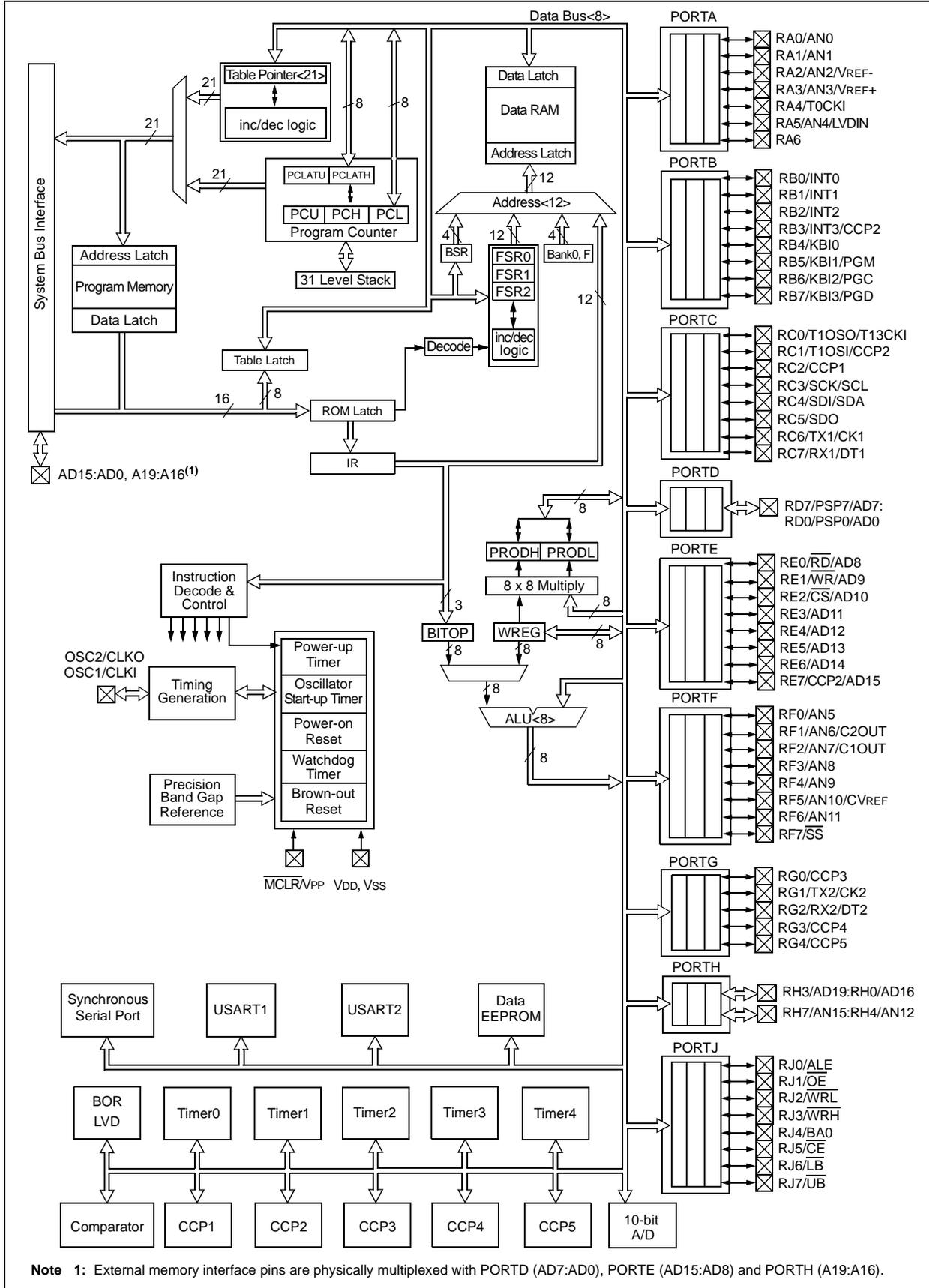
Note 1: External memory interface pins are physically multiplexed with PORTD (AD7:AD0), PORTE (AD15:AD8) and PORTH (A19:A16).
