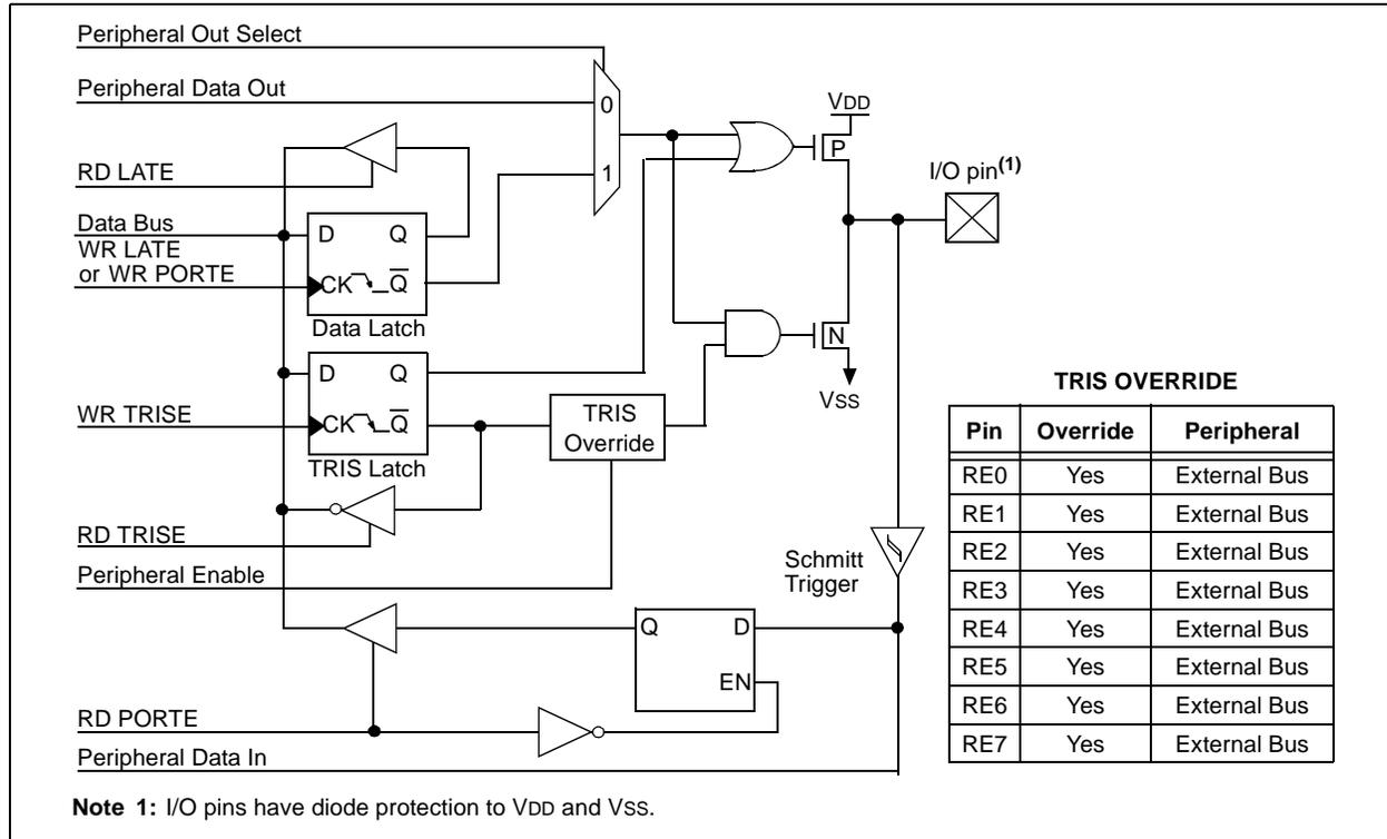
**FIGURE 10-12: PORTE BLOCK DIAGRAM IN SYSTEM BUS MODE**
