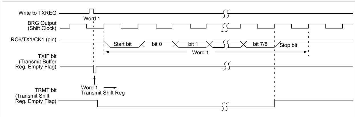
**FIGURE 18-3: ASYNCHRONOUS TRANSMISSION (BACK TO BACK)**
