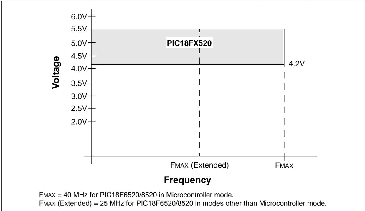
FIGURE 26-2: PIC18LF6520/8520 VOLTAGE-FREQUENCY GRAPH (INDUSTRIAL)
