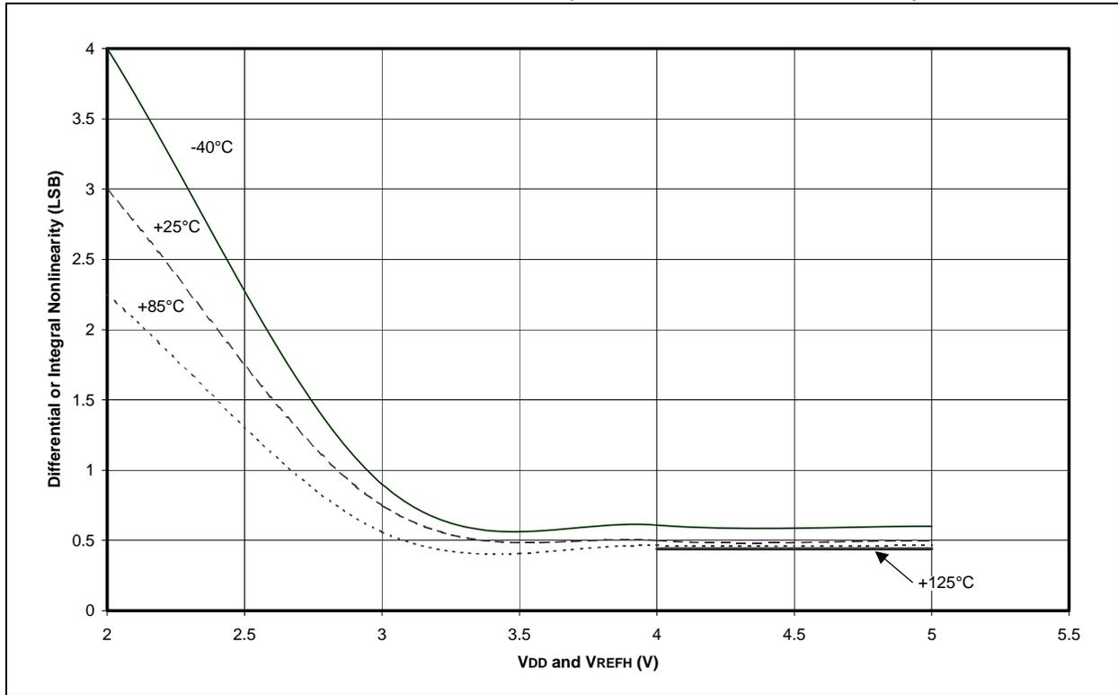
FIGURE 27-26: A/D NONLINEARITY vs. VREFH (VDD = 5V, -40°C TO +125°C)
