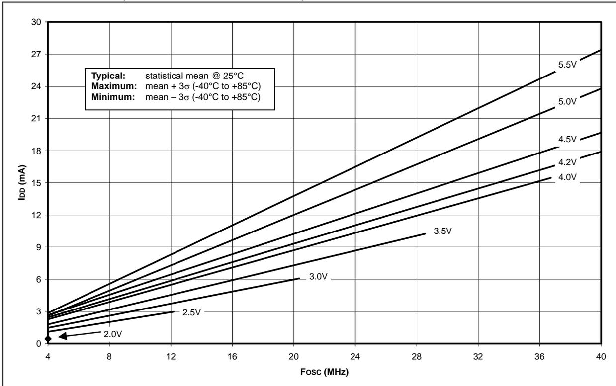
**FIGURE 27-24: MAXIMUM I<sub>DD</sub> vs. Fosc OVER V<sub>DD</sub> (HS/PLL MODE) EXTENDED (PIC18F8520 DEVICES ONLY)**
