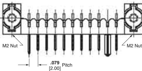
**2 mm Plug Assembly with Nut Plates**
