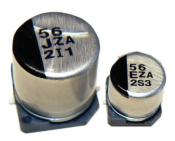
Rated for 105°C, type HZA combines the advantages of aluminum electrolytic and aluminum polymer technology. These hybrid capacitors have the ultra-low ESR characteristics of conductive aluminum polymer capacitors packaged in a V-chip, SMT case with high capacitance and voltage ratings
