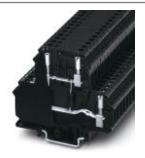
Double-level modular terminal block with suppressor diode as surge protection between both levels, nominal voltage: 60 V AC, for mounting on NS 32 or NS 35/7.5, closed housing, terminal width: 6.2 mm, terminal height: 68 mm
