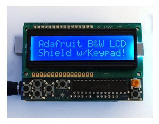
This shield is perfect for when you want to build a stand-alone project with its own user interface. The 4 directional buttons plus select button allows basic control without having to attach a bulky computer.
