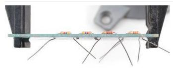
Make sure the resistors all sit nice and flat against the PCB.
