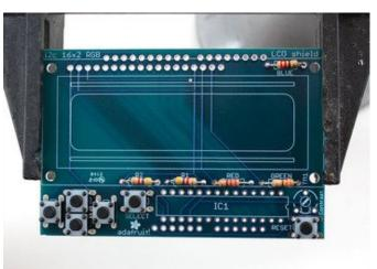
Next up we will place the buttons. These buttons are useful to send a signal to the Arduino (say if you have a basic menu system). We have a 4-way 'direction pad' for up/down/left/right input and a button to the right called SELECT. These 5 buttons should be able to make 'talking' back to your project easy. These are connected to the I2C port expander chip so they require no extra pins on the Arduino, our library does the work of reading whether they are pressed.
