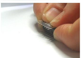
We're nearly done! Now we will place the I2C port expander chip. Double check that it has the MCP23017-E/SP marking on it. This is a 16-pin expander chip, that uses the i2c bus. That means you can send it commands using the i2c pins on an Arduino and control 16 more digital pins! 5 of those pins go to the buttons, 6 go to the LCD control and 3 are used for the backlight (the remaining 2 are unused).
