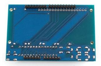
Flip over the shield and place it flat on the table so the long leads of the header stick out.
