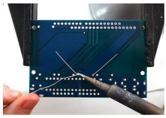
With your soldering iron heated up and ready, solder in both leads of the resistor. To do this, heat up the round ring pad and the wire lead at the same time for 2 or 3 seconds, then dip the end of the solder into the heated joint to melt it in.
