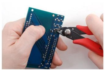
Solder all of the header pins. Even though they aren't used for passing signals, they will make the mechanical connection to the Arduino strong.
