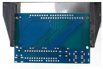
Flip over the PCB and check that all the legs for the buttons are sticking out.
