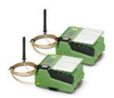
Wireless-MUX set, two modules with 16 digital inputs and outputs and 2 analog inputs and outputs (0 ... 20 mA, 0 ... 10 V) each, omnidirectional antennas with 1.5 m cable, 24 V DC supply voltage
